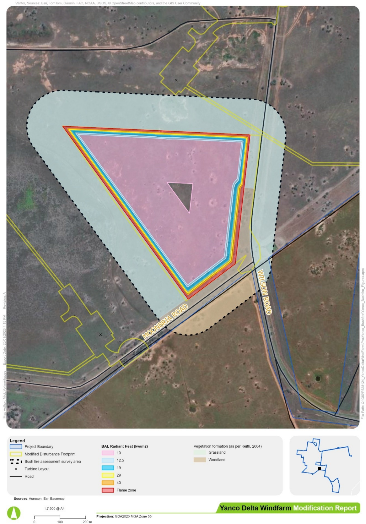
Figure 4-9 Spark-BAL assessment for temporary workers accommodation (TWA)
