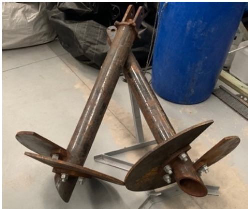
Figure 35: Typical screw anchor shaft with helix and pivot point (Credit: Blue Harvest 2025).
