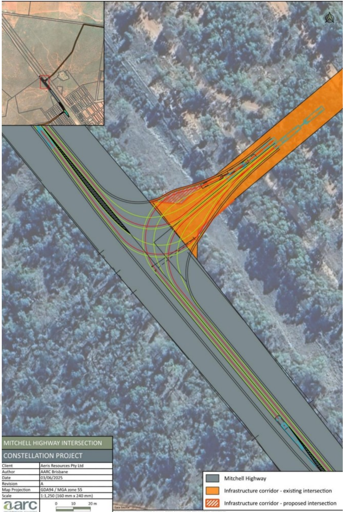
Figure 1: Intersection of haul road with eastern side of Mitchell Highway
