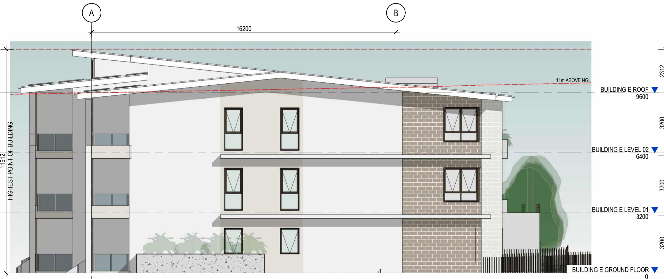
4 BUILDING E - WEST ELEVATION 1:100
