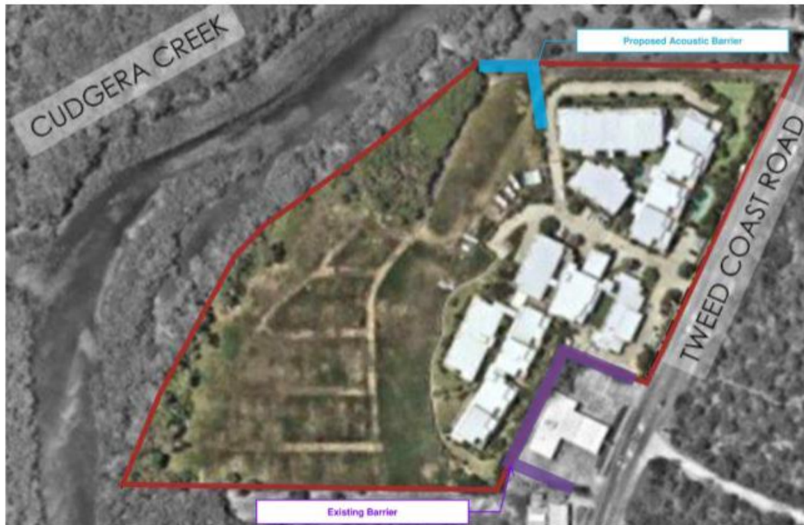
Figure 6-12 | Acoustic Barrier Locations (Source: ADP Consulting)
