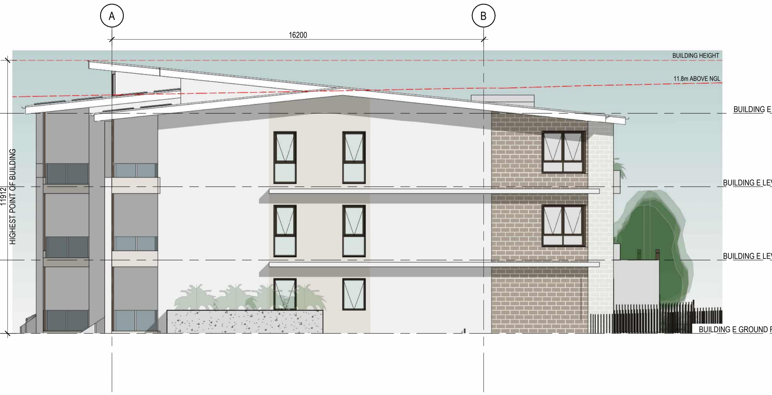
4 BUILDING E - WEST ELEVATION 1:100
