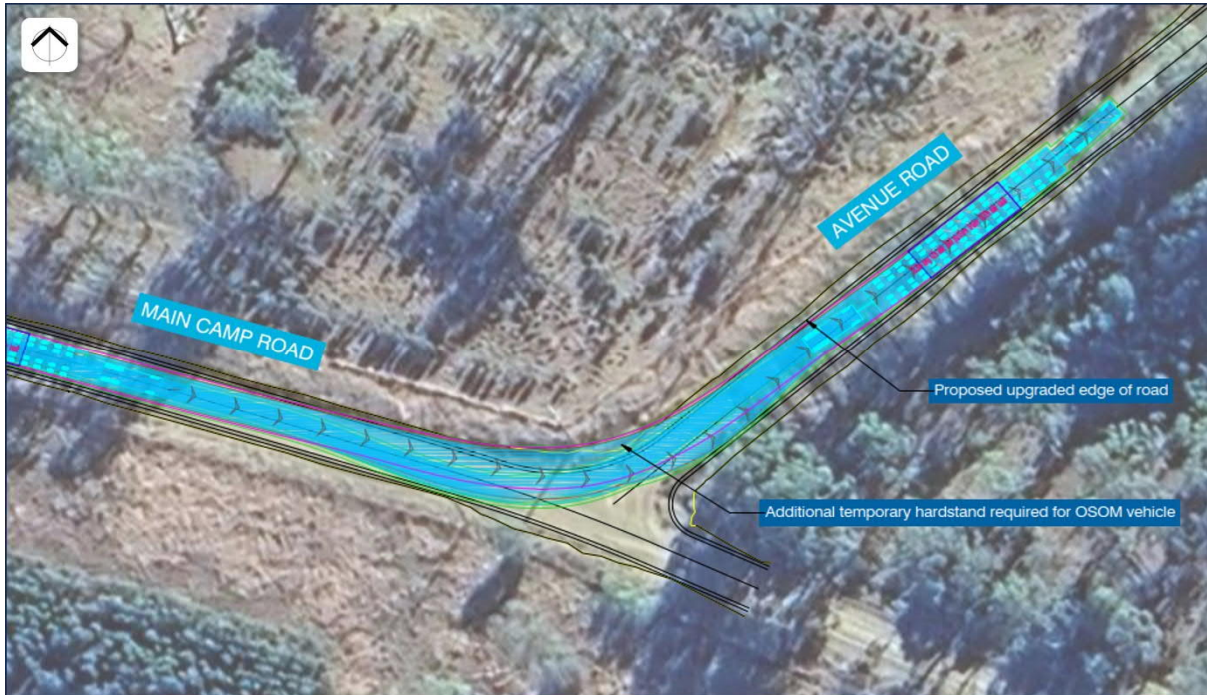
Figure 26 OSOM Transport Vehicle Swept Paths – Main Camp Road / Avenue Road [Source: EMM Consulting Pty Ltd]
