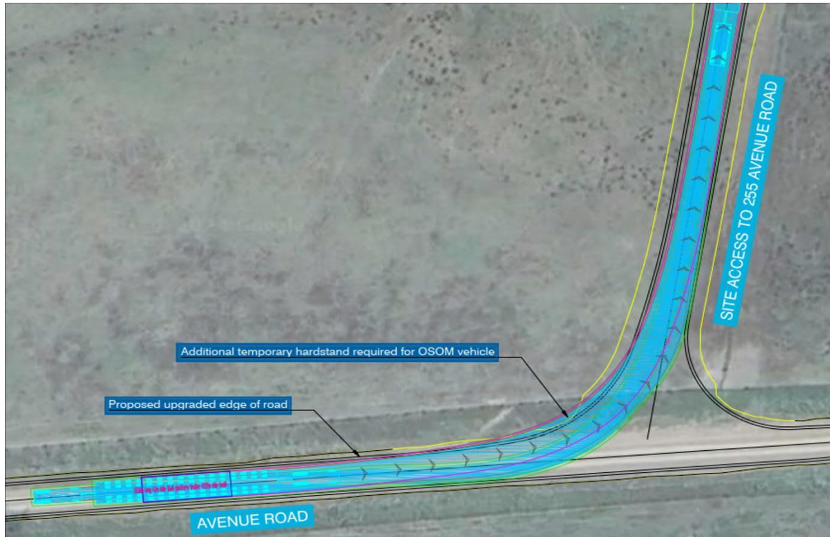
Figure 28 OSOM Transport Vehicle Swept Paths – Avenue Road / Site Access SA2 [Source: EMM Consulting Pty Ltd]
