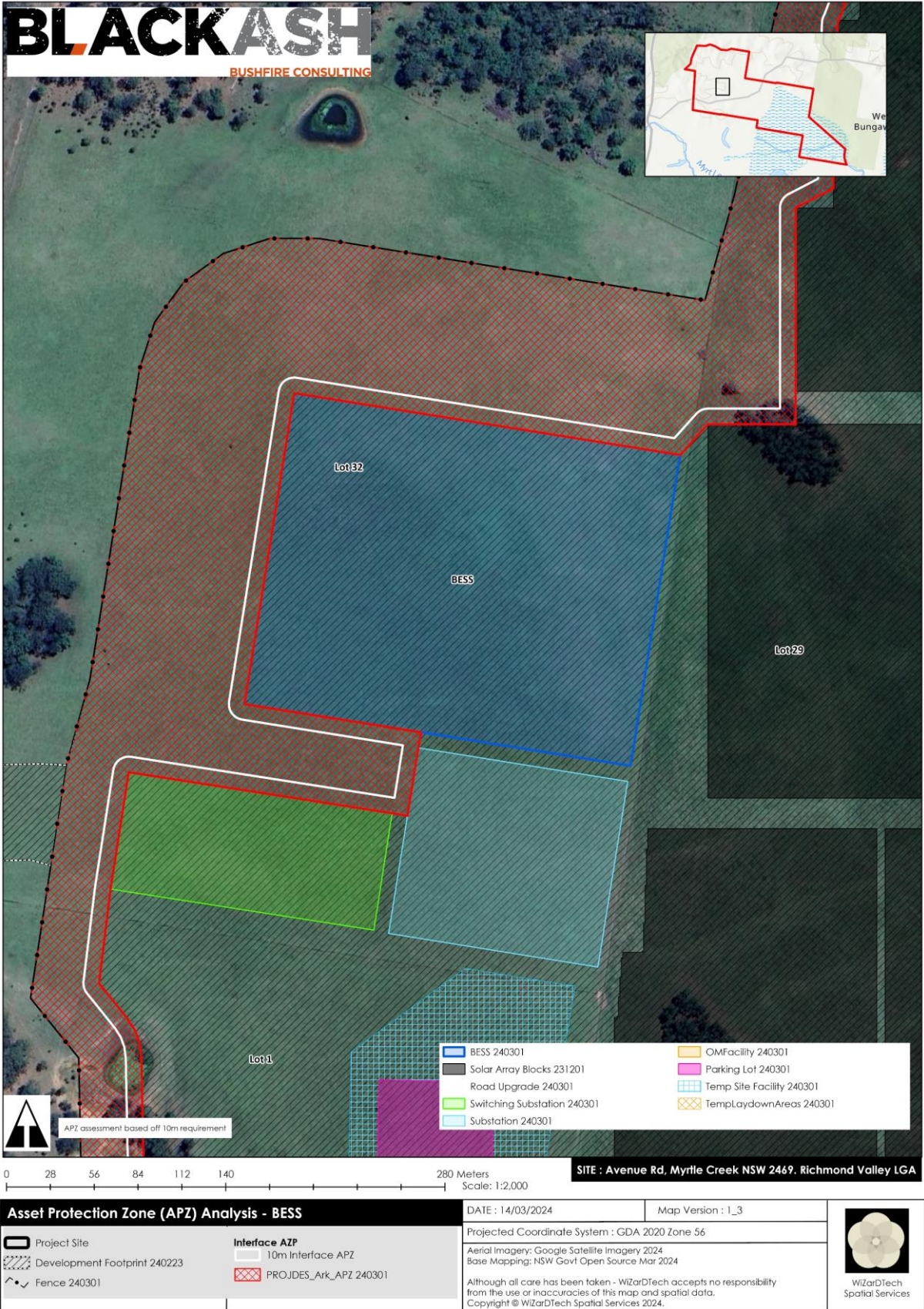
Figure 25: APZ map around critical infrastructure (note: transmission corridor to west of switching substation will also be maintained to APZ standards)
