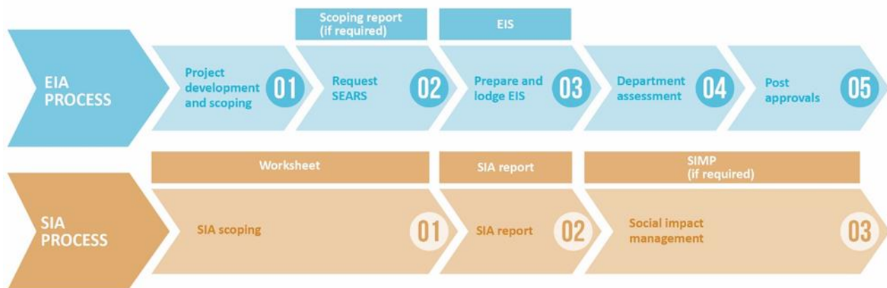
Figure 2.1 SIA and EIA Process
