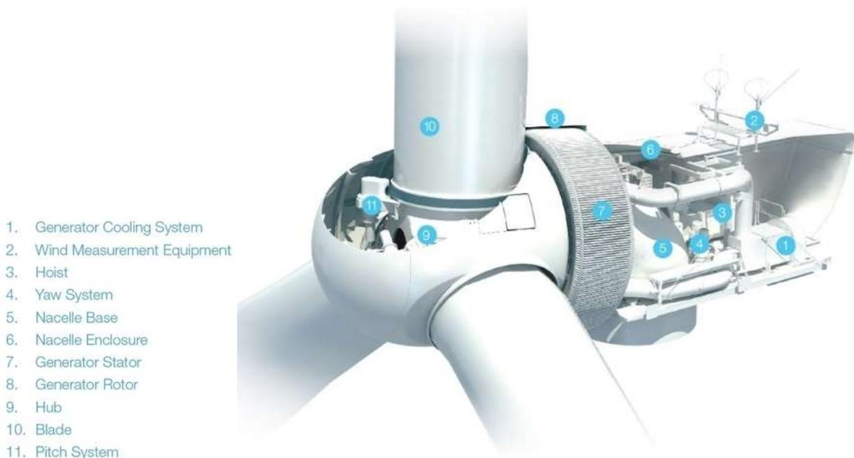
Figure 3-1: Wind turbine nacelle cut-away
