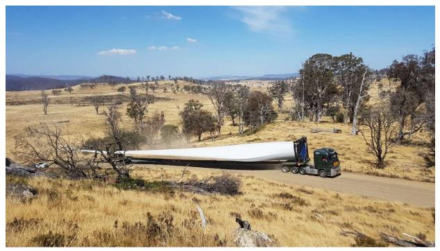
Figure 3-4: Transport of a 68.6 metre wind turbine blade to site (Cattle Hill Wind Farm 2019)
