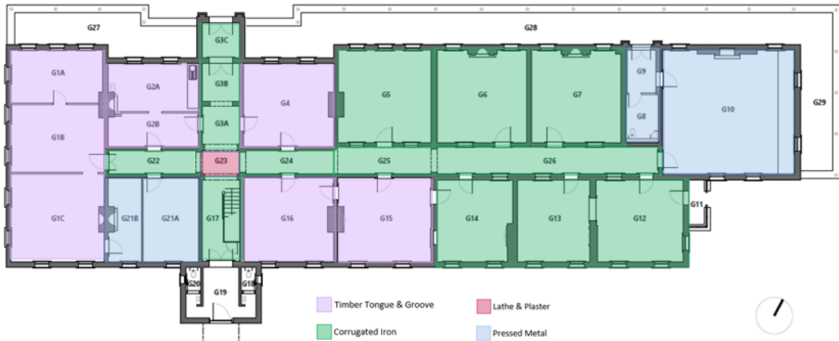
Figure 4.29: Ground Floor Ceiling Type Plan of the CME Building
