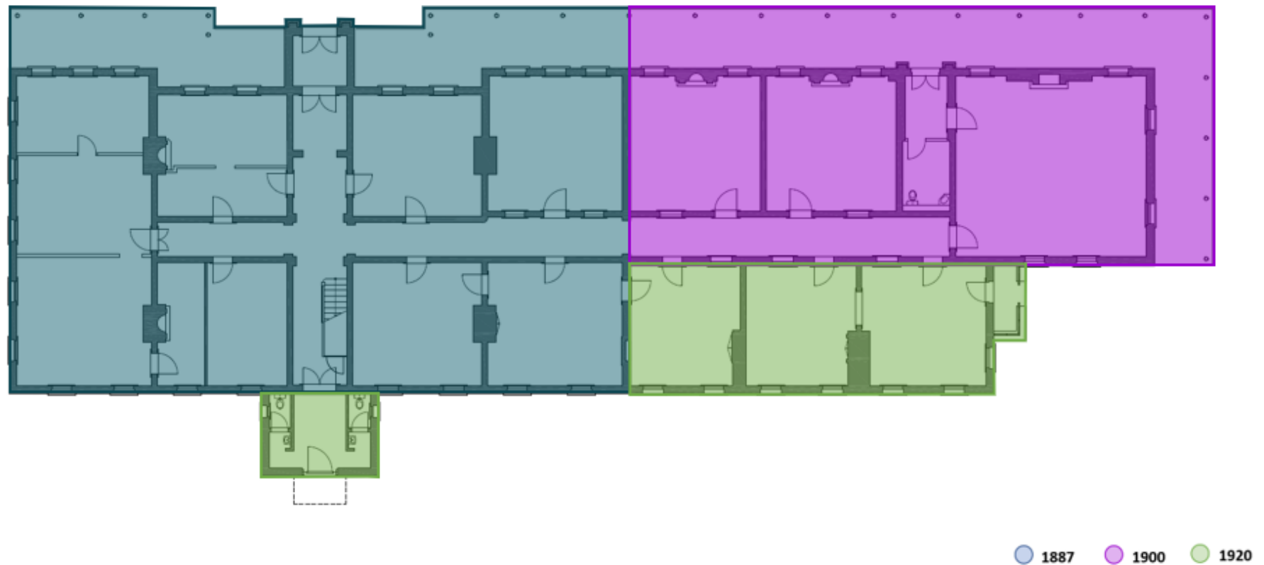
Figure 4.16: Ground floor plans of the CME building with the three main phases of construction. (Source: Rappoport & Caldis Cook Group, 1997 with Curio additions)
