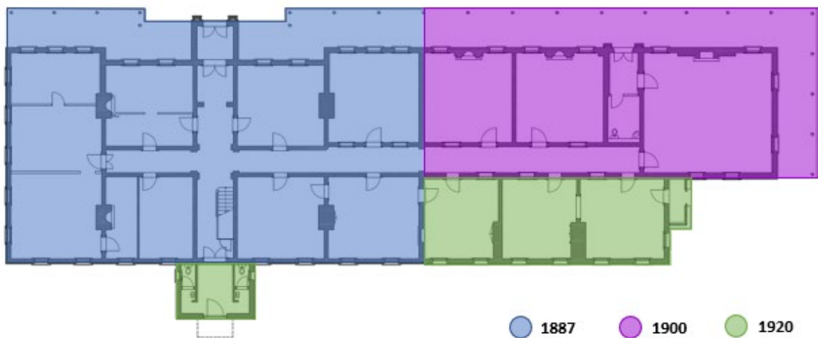
Figure 2.12: Ground floor plan of the CME Building showing the three main phases of construction. Source: Curio 2022
