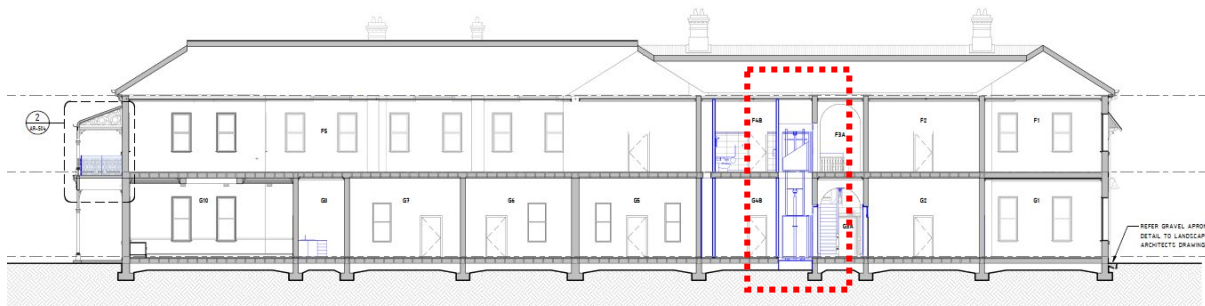
Figure 8.4: Section showing the proposed lift. The chosen model has a reduced lift overrun that will allow the lift to be contained without the building. Source: CCG Architects, 2022.
