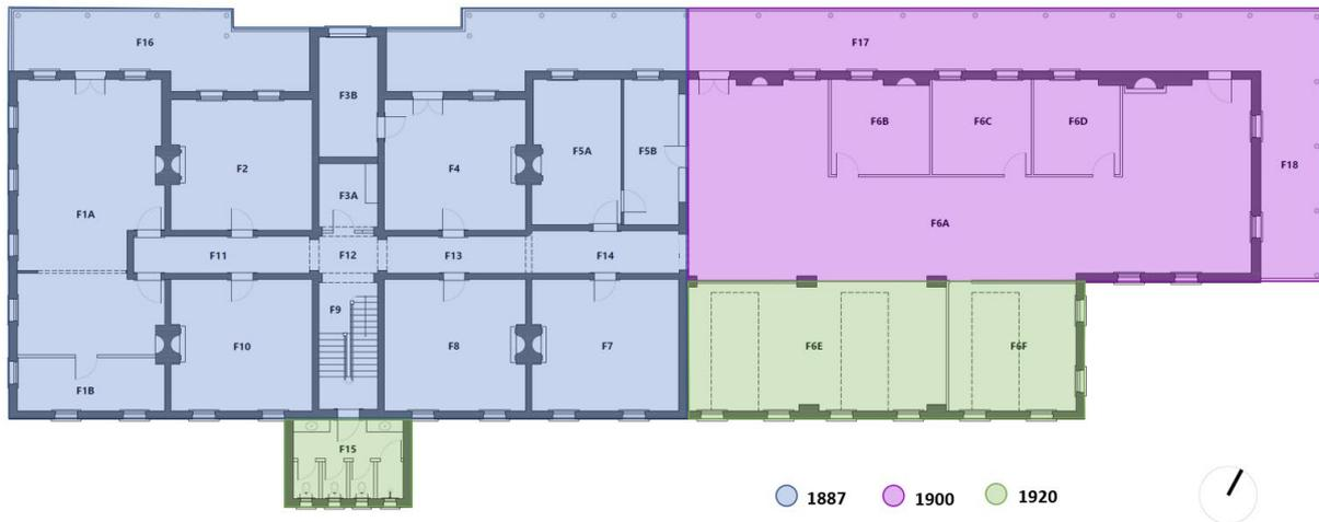
Figure 3.6: Phases of Construction: First Floor Plan. Source: Curio Projects, 2022.
