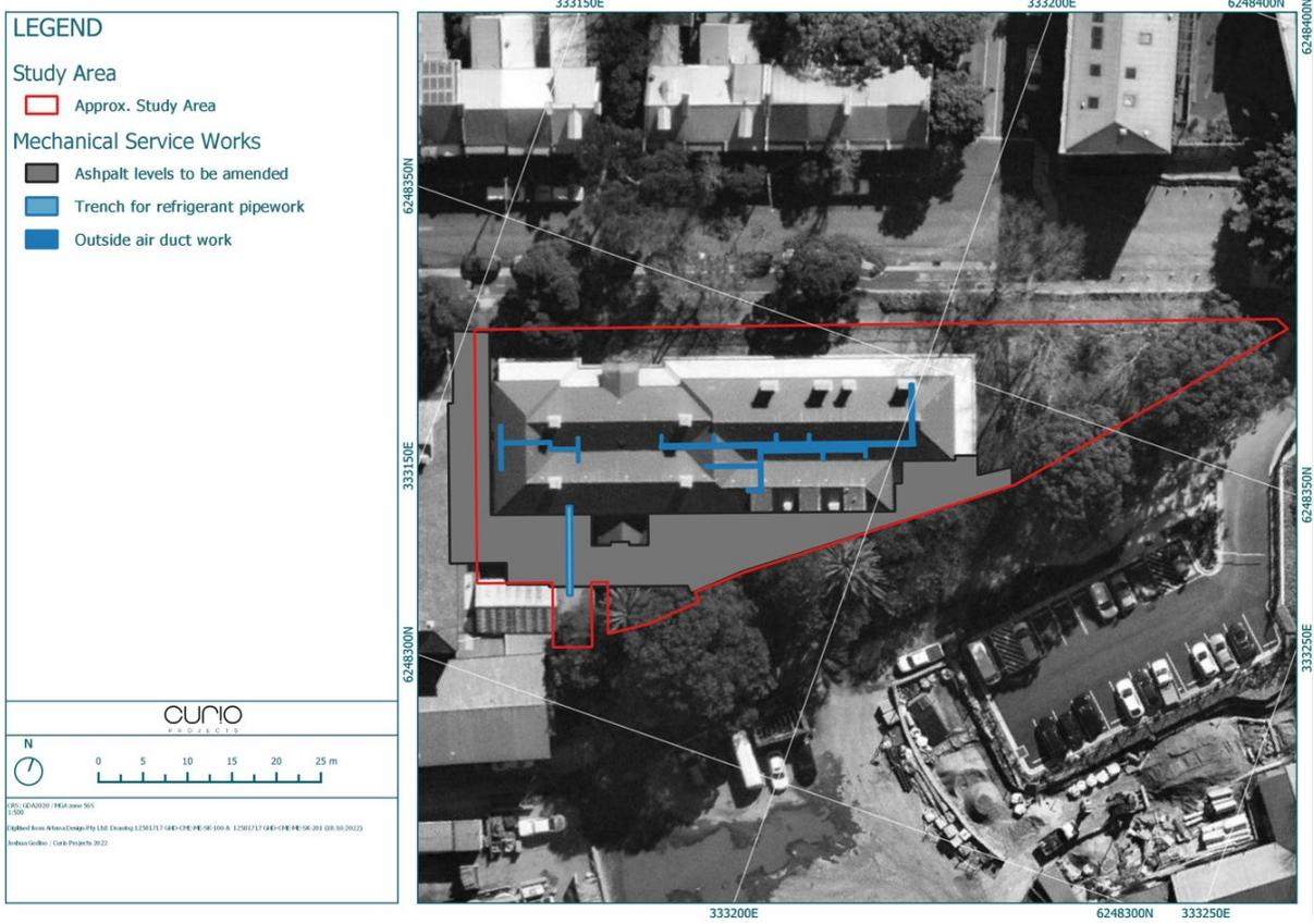
Figure 6-5: Mechanical services scope of work
