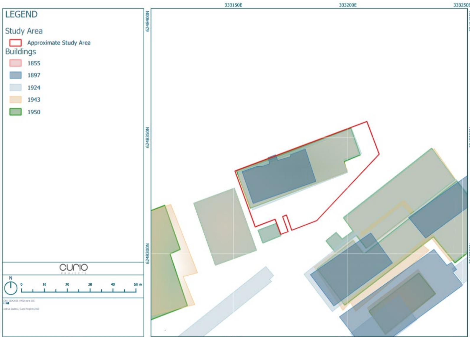
Figure 5-8: Compilation overlay showing identified extension of the CME building from the 1850s to 1950s. Source: Curio 2022
