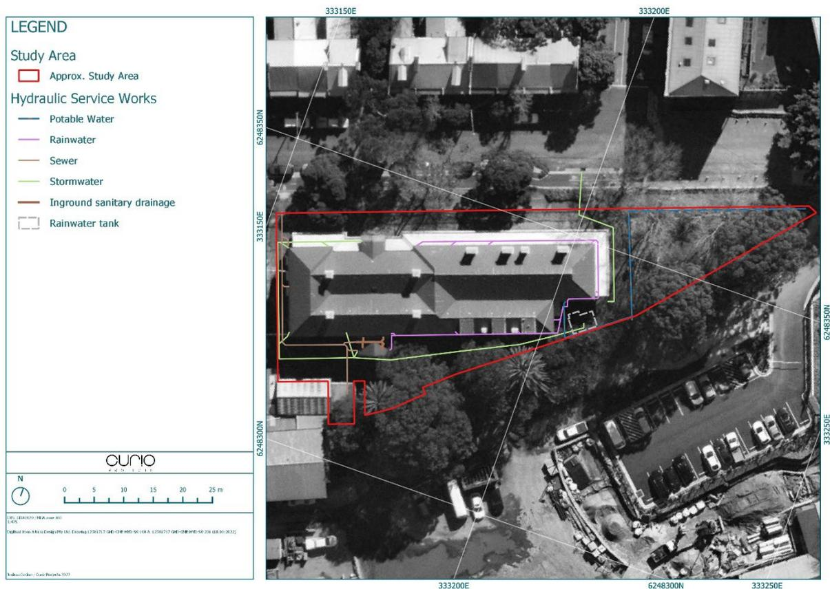
Figure 6-4: Hydraulic services scope of work
