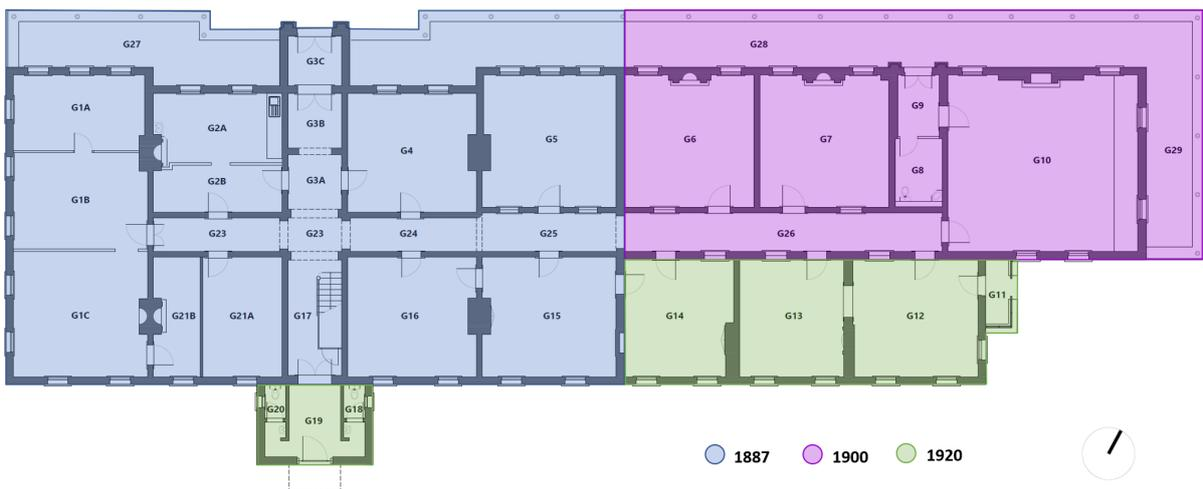
Figure 3.5: Phases of Construction: Ground Floor Plan. Source: Curio Projects, 2022.
