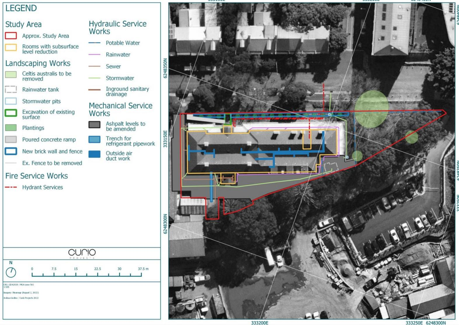
Figure 6-6: Summary of Proposed Ground Disturbing Works
