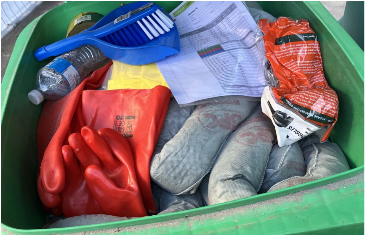
Spill kit fully stock including absorbent sock and safety equipment.
