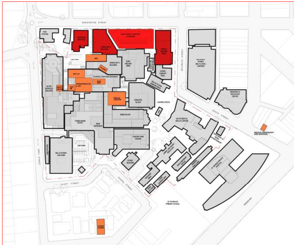
Figure 1.2 The Existing Site: Stage 3 Works with Adaptive Re-use in Orange and Demolition in Red (Source: Jacobs)
