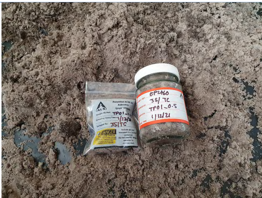
Plate 5 – Representative image of Soil material observed during SCA (EP Risk 2021): sand, fine to medium grained, grey, slightly moist, loose consistency.
