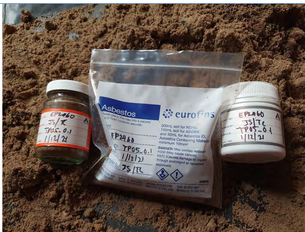
Plate 6 – Representative image of Soil material observed during SCA (EP Risk 2021): Gravelly sand, medium grained, angular to sub-angular gravels, light brown, slightly moist and loose.
