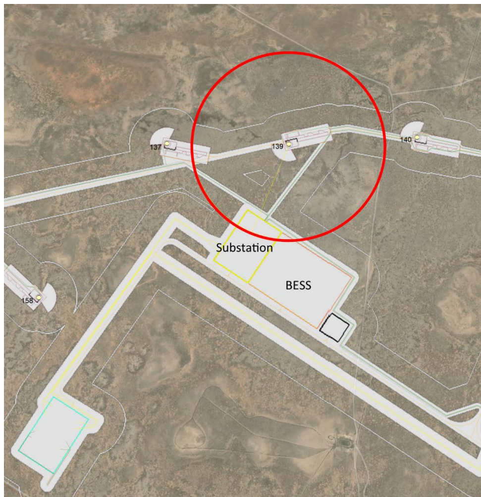
Figure 31: Example Maximum Ice Throw Hazard Ranges for WTG No. 139
