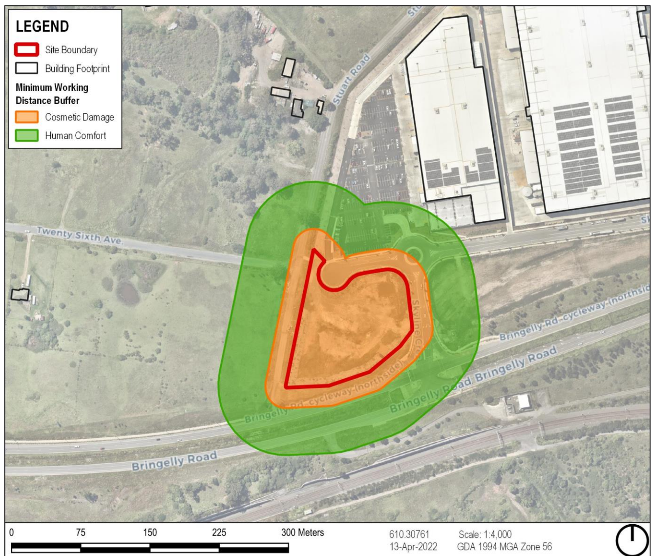
Figure 4 Construction Vibration – Large Hydraulic Hammer
