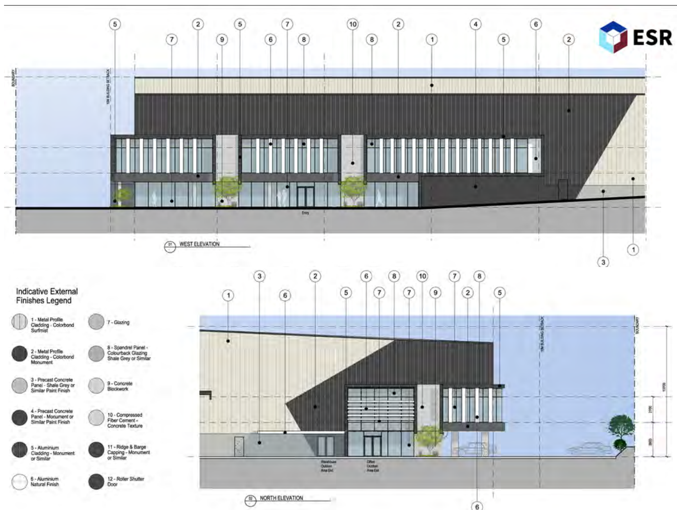
OFFICE ELEVATION + INDICATIVE EXTERNAL FINISH - SBA ARCHITECTS
