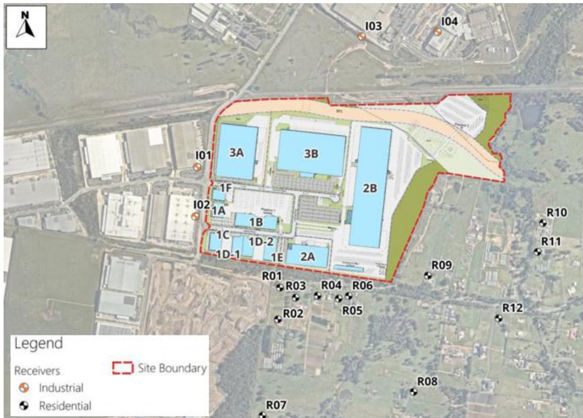
Figure 59: Sensitive receivers in relation to OEE (Source: RWDI)
