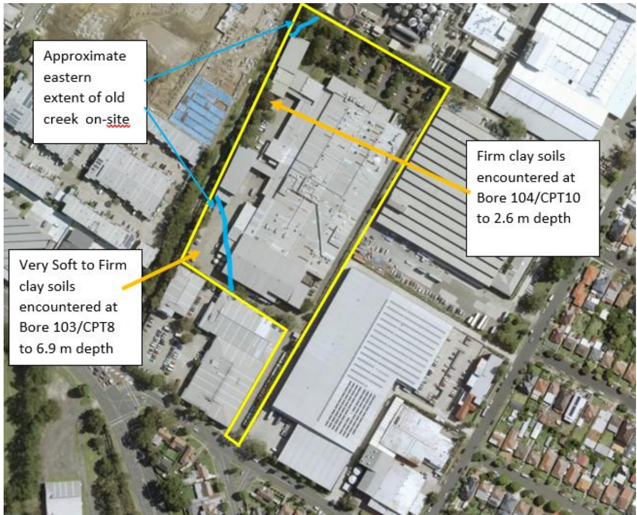
Figure 6. Approximate Extent of Old Creek Alignment on-site and Test Location where softer soils were encountered.
