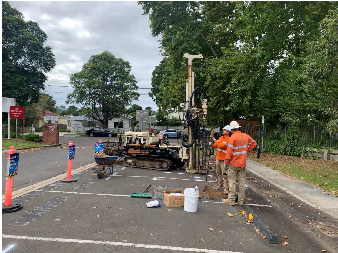
Photograph 1: Delineation sampling of soils surrounding BH01 advanced during the ESA (Cardno, 2022) using a hand auger and Geoprobe 7822DT
