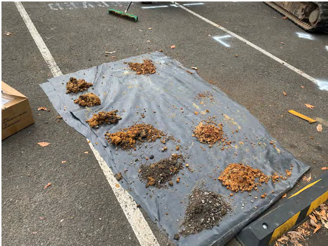
Photograph 2: Spoil from BH01S2 which was advanced to delineate contamination from BH01
