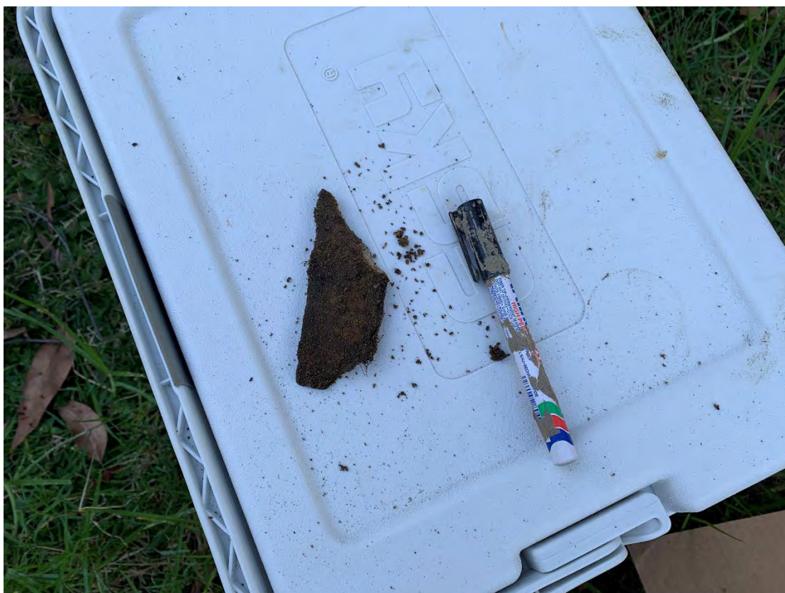
Photograph 15: Bonded asbestos fibre cement fragment observed in TP23 (TP23_0.3_PACM)
