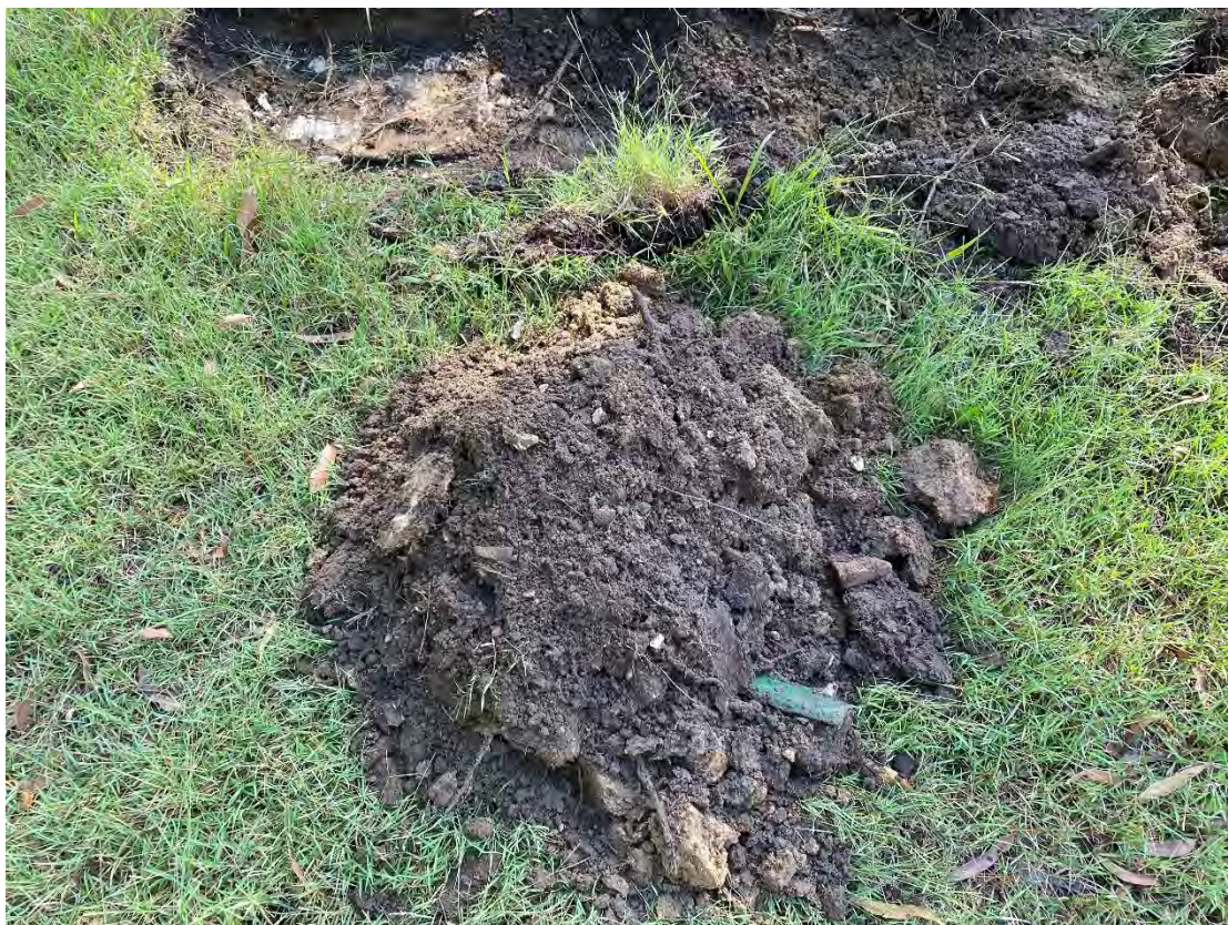
Photograph 13: Spoil from TP20, note bonded asbestos fragment (TP20_PACM_20_0.1)
