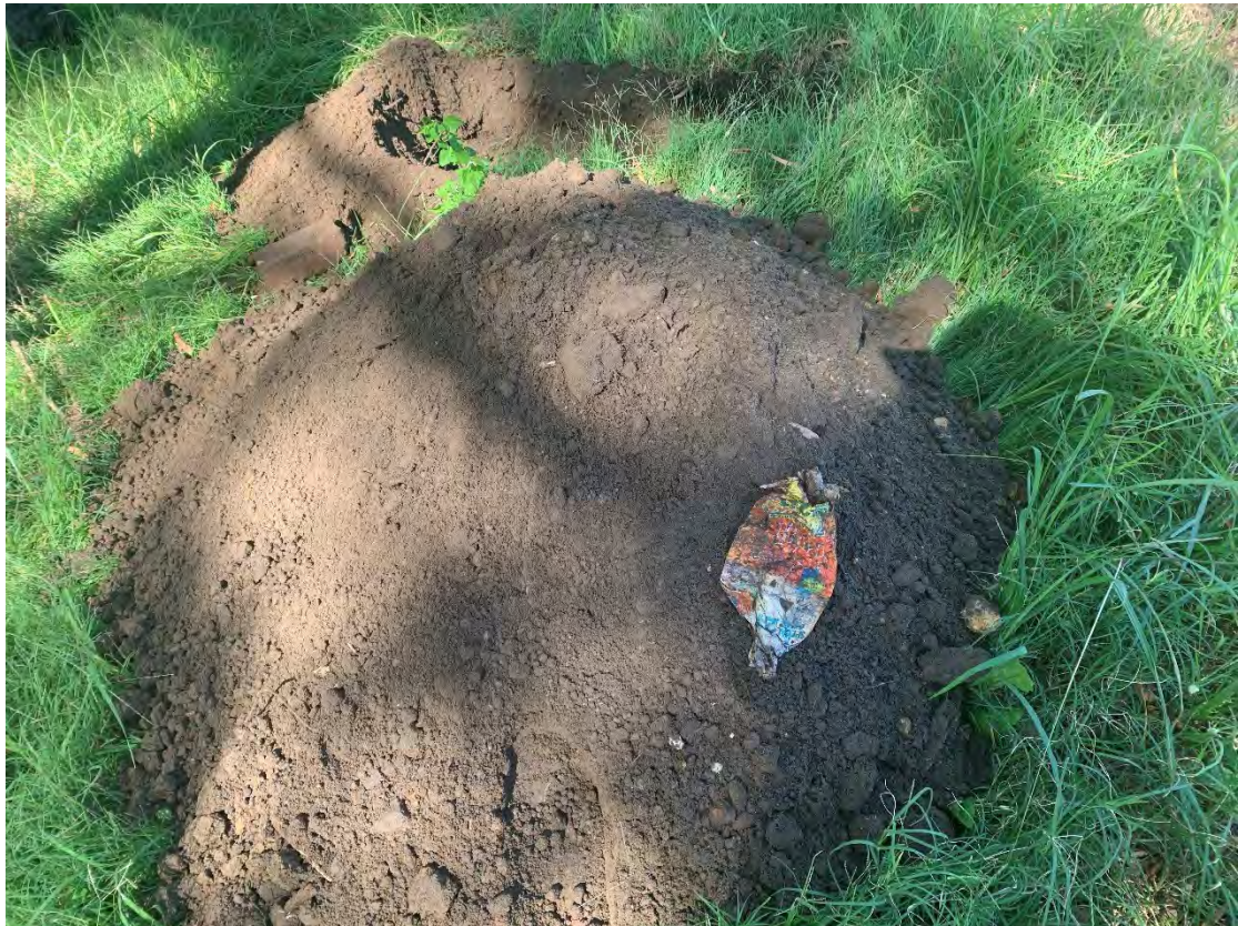
Photograph 9: Spoil from TP11 advanced in the western fill bank within the Site, note plastic and brick
