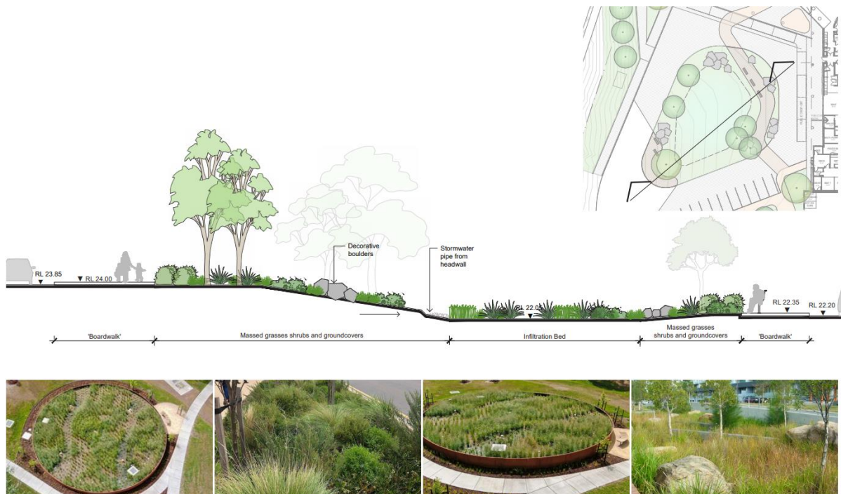
Figure 53 – Section through the proposed Central Drop-Off Raingarden (Site Image)
