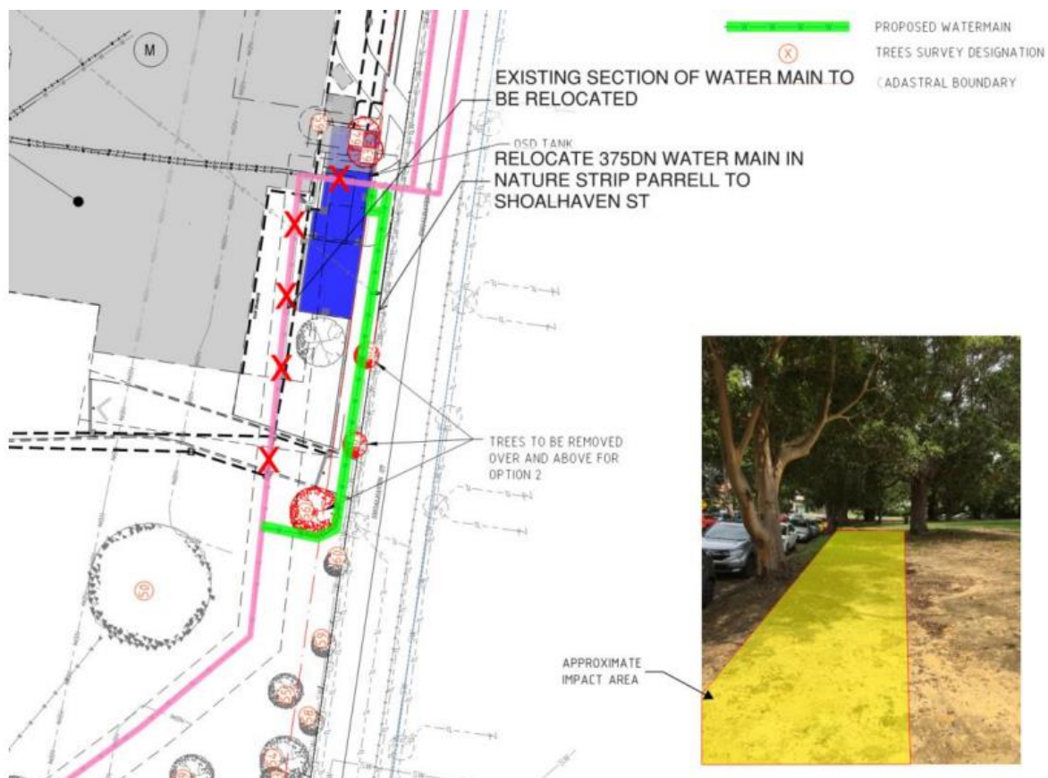
Figure 66 - Proposed Shoalhaven Water Main Relocation - shown in green (Jacobs)
