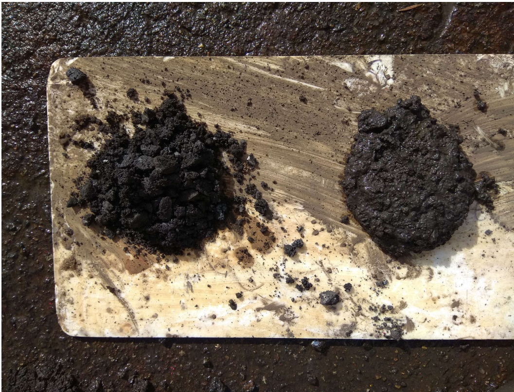
Photo 4: Typical FILL retrieved from the boreholes (11/07/2022)
