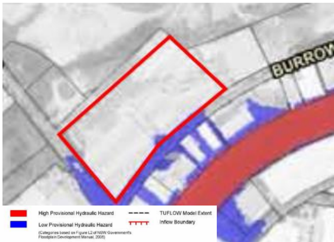
Figure 7.7. M5 EIS - 1% AEP Provisional Flood Hazard
