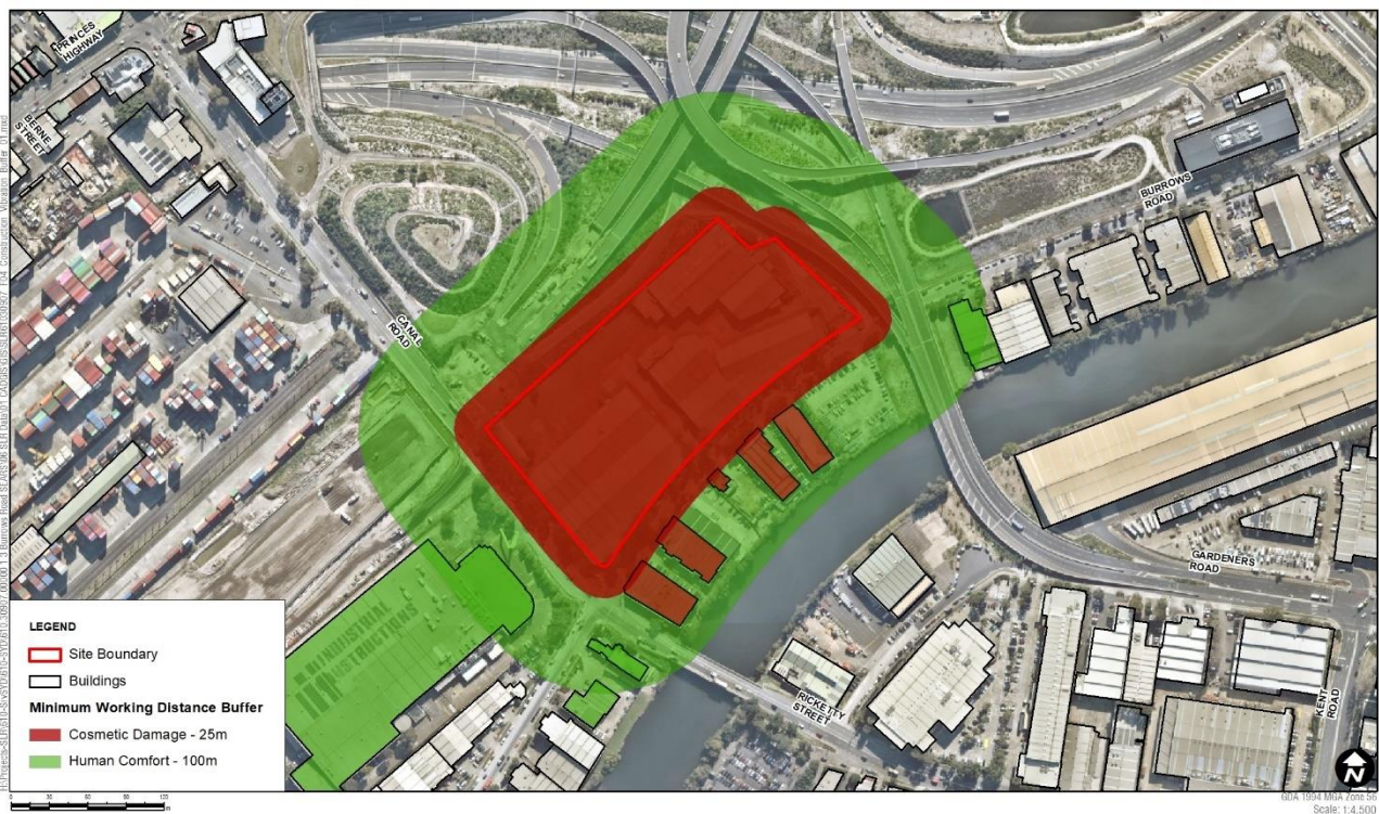
Figure 7 Construction Vibration – Large Vibratory Roller
