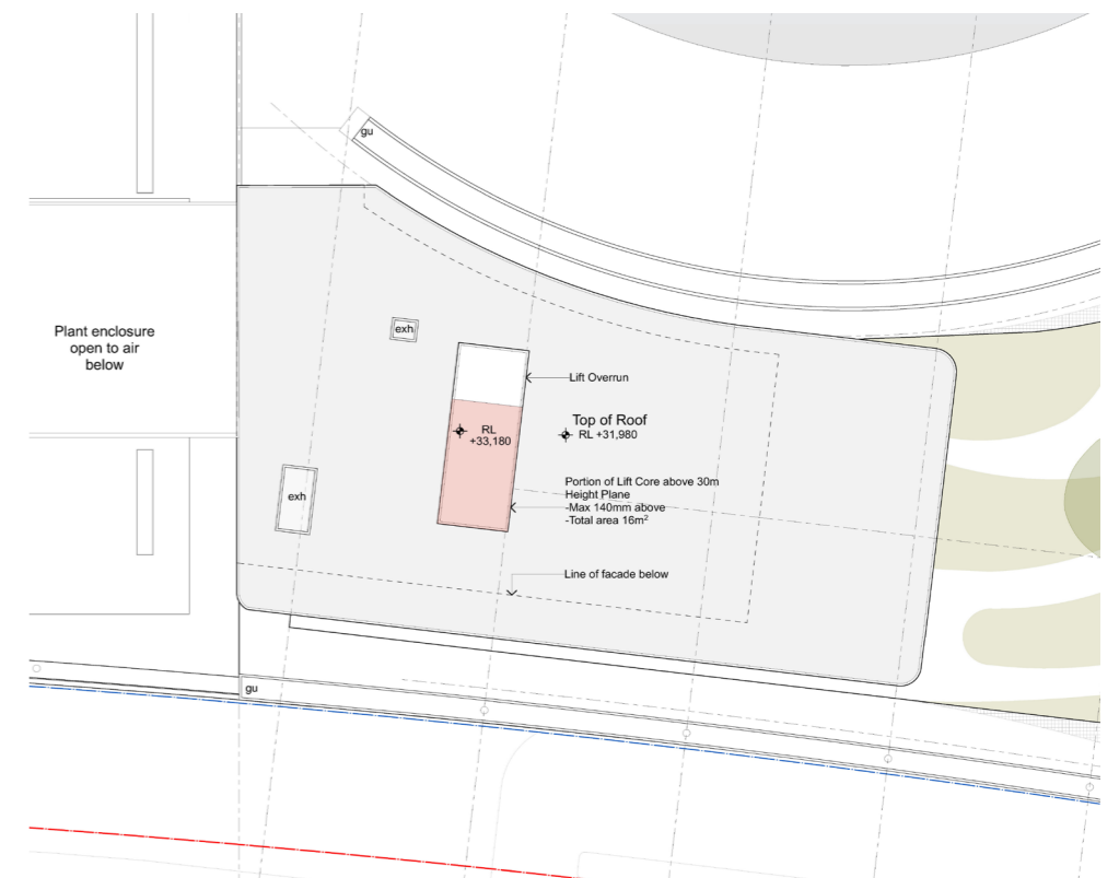
Roof plan indicating area of lift over run that exceeds 30 m height above existing ground
