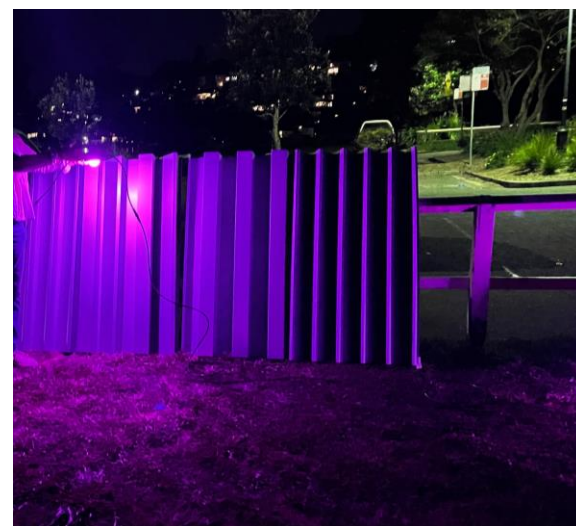
LED Dots close to horizontal – promotes illumination of panel and nodes are still visible
