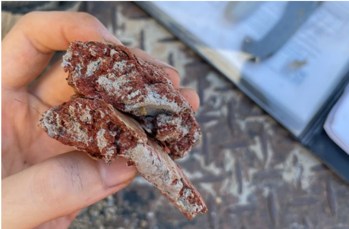
Photo 7 - Typical RESIDUAL (CLAY) unit
