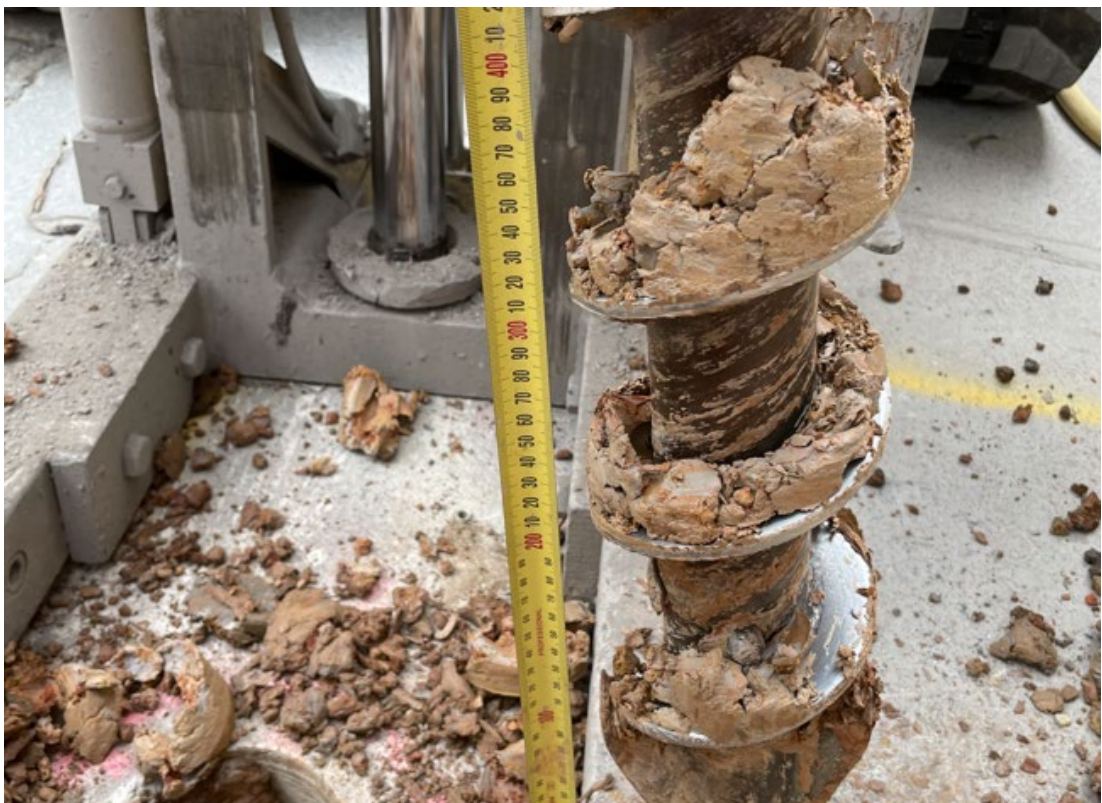
Photo 8 - Typical RESIDUAL (CLAY) unit at BH02
