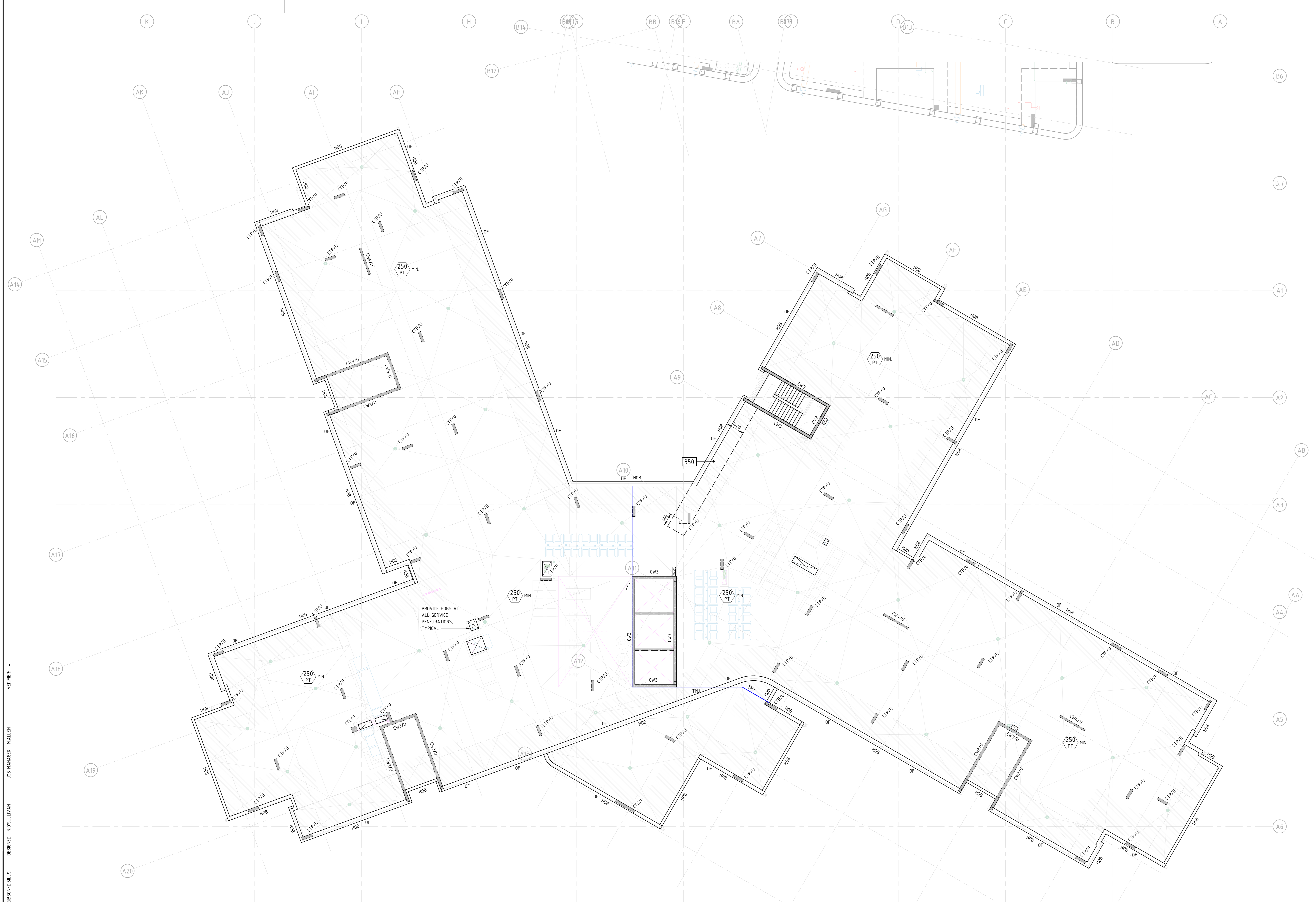
BUILDING A - ROOF PLAN ROOF SLAB TO BE DESIGNED AS WATERTIGHT SLAB, MINIMUM 20MPa PRESTRESS AND MESH TO ALL AREAS
