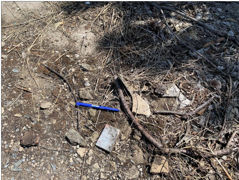
Photo 18: Fibro fragments on the surface of the hardstand in the south-western portion of the hardstand.
