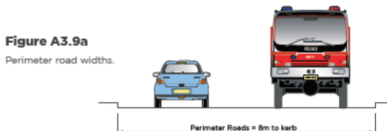
Figure 9 PBP Perimeter requirements
