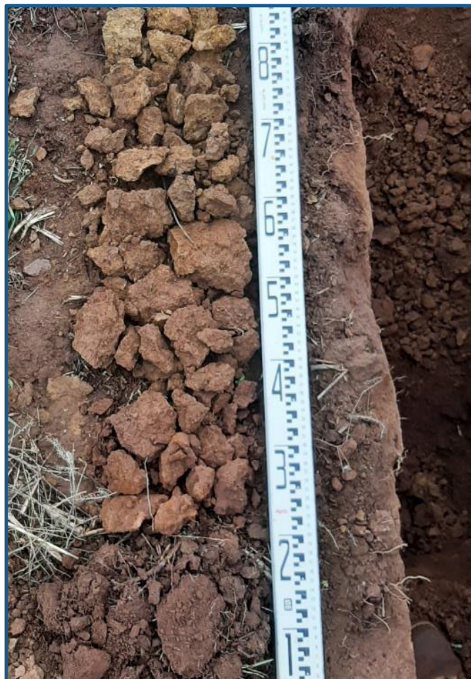
Images 7 (left) & 8 (right): The gradational soil profile of the Red Friable Soil consists of 15 cm of red-brown, well structured, friable clay loam topsoil (A Horizon) overlying a transitional subsoil layer of red-brown, well structured, friable, light clay (B1 Horizon), which in turn overlies a dull red-brown, moderately structured, semi-friable, medium clay subsoil (B2 Horizon); deeper subsoil layers consist of medium to heavy clay with yellow colouration.
