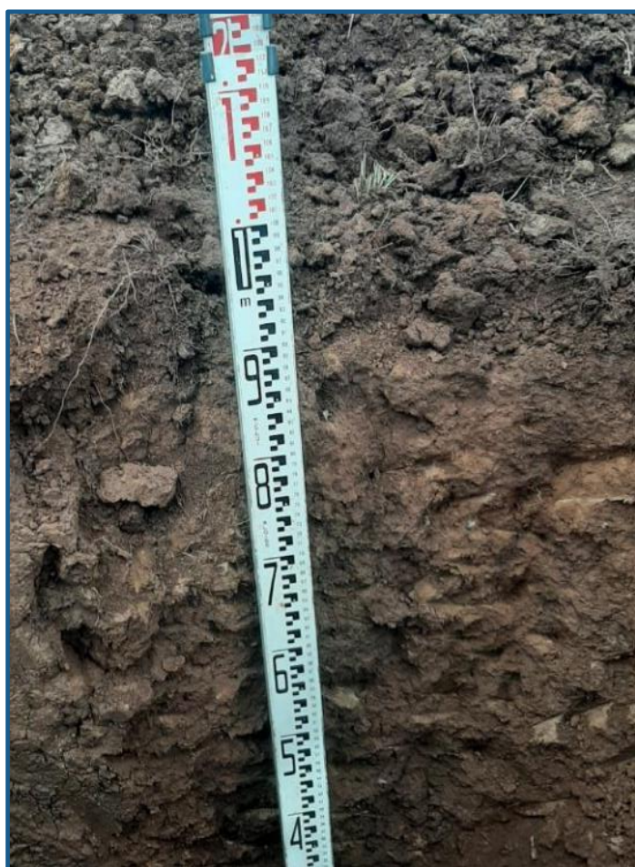
Images 10 (left) & 11 (right): The Plex Brown Plastic Soil consists of a shallow (7 cm) weekly structured, sandy clay loam topsoil (A Horizon) overlying a thin (2 cm) poorly structured, slightly cemented layer (B1 Horizon) which, at a depth of 9 cm, rapidly transitions into a poorly structured, dense, tough, plastic, medium to heavy clay subsoil (B2 Horizon) which extends to depth (100+ cm).
