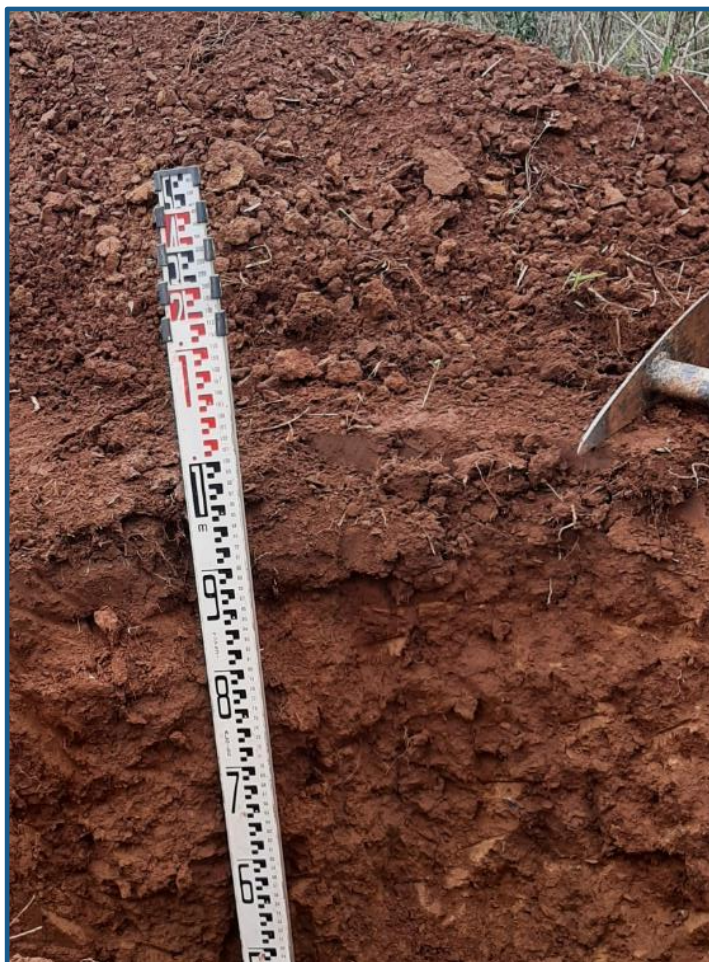
Images 7 (left) & 8 (right): The gradational soil profile of the Red Friable Soil consists of 15 cm of red-brown, well structured, friable clay loam topsoil (A Horizon) overlying a transitional subsoil layer of red-brown, well structured, friable, light clay (B1 Horizon), which in turn overlies a dull red-brown, moderately structured, semi-friable, medium clay subsoil (B2 Horizon); deeper subsoil layers consist of medium to heavy clay with yellow colouration.
