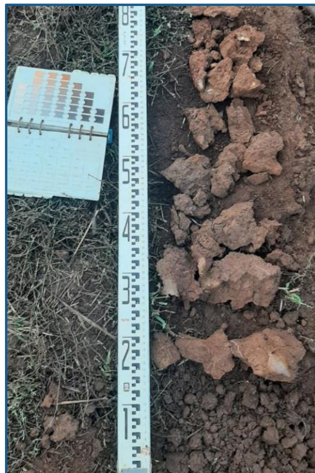
Images 10 (left) & 11 (right): The Plex Brown Plastic Soil consists of a shallow (7 cm) weekly structured, sandy clay loam topsoil (A Horizon) overlying a thin (2 cm) poorly structured, slightly cemented layer (B1 Horizon) which, at a depth of 9 cm, rapidly transitions into a poorly structured, dense, tough, plastic, medium to heavy clay subsoil (B2 Horizon) which extends to depth (100+ cm).
