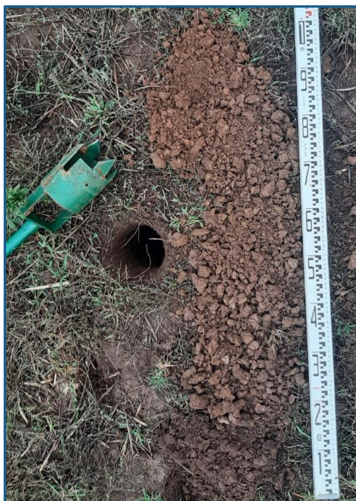
Image 2 (left): The soil profile was examined and logged in 2 soil profile inspection pits excavated on the site.
