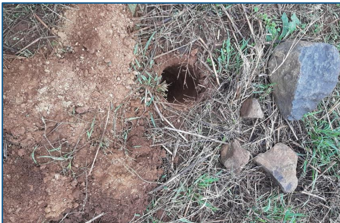
Image 5: The Rocky Soil consists of friable red-brown sandy clay loam and Ordovician sedimentary rock.
