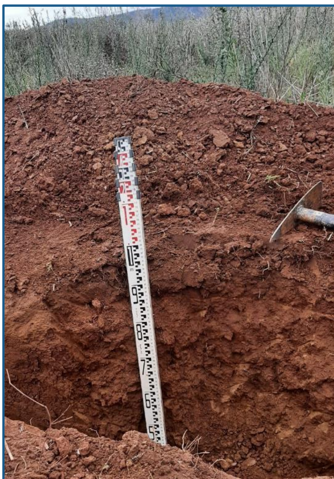
Image 2 (left): The soil profile was examined and logged in 2 soil profile inspection pits excavated on the site.
