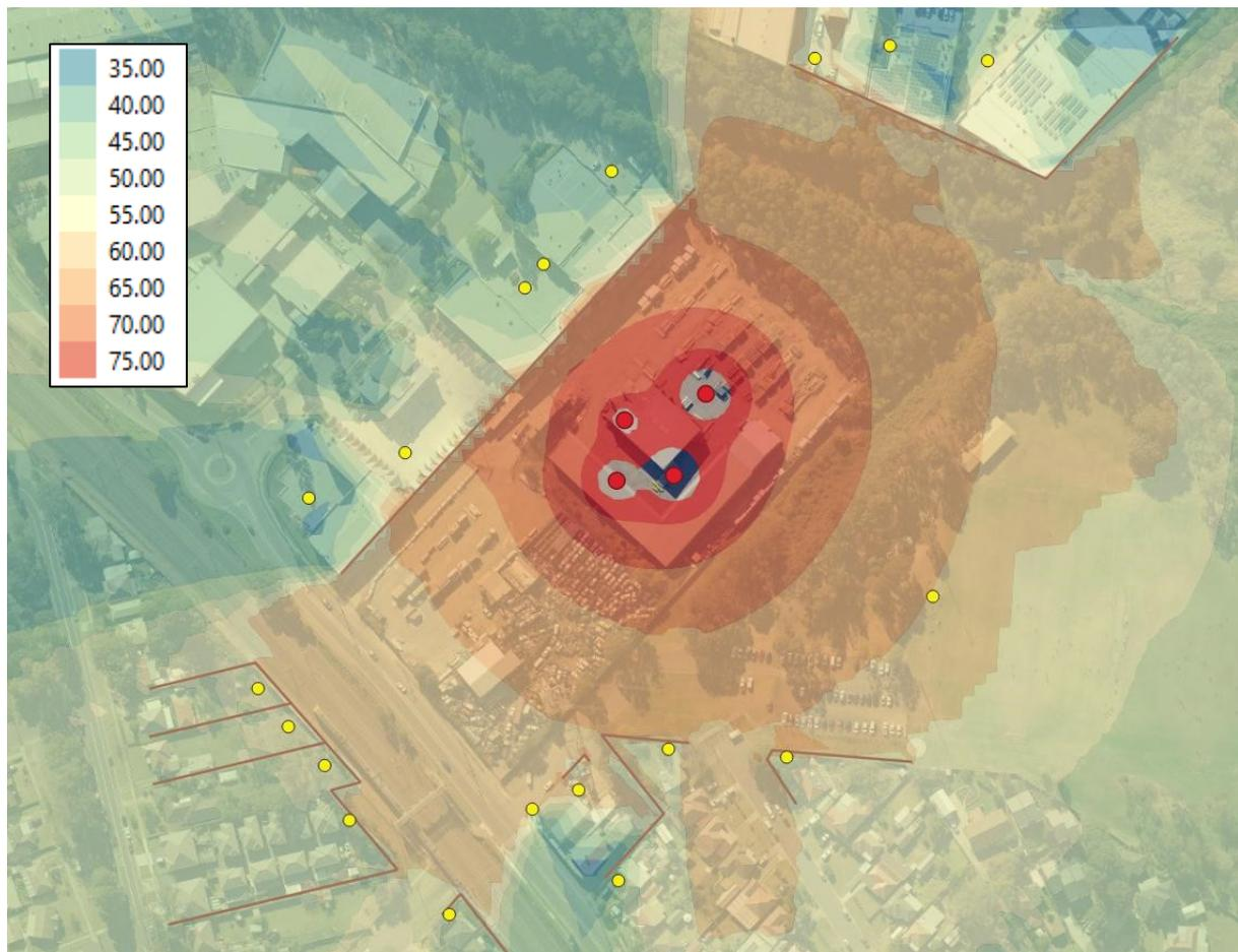
**Figure 25 Predicted Noise Contours – Construction Scenario 2,  $L_{Aeq}$  (15 minute)**
