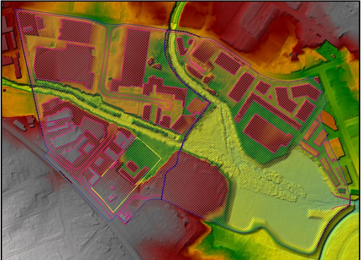
**Figure 6 : Existing Hec-Ras 2D Model Layout (from Geometric Data Viewer)**
