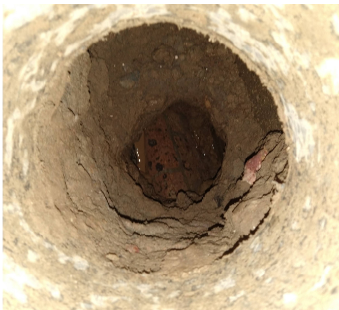
Photo D3 – View down Borehole BH1003 at the borehole refusal depth, showing a section of mortared brick rubble.
