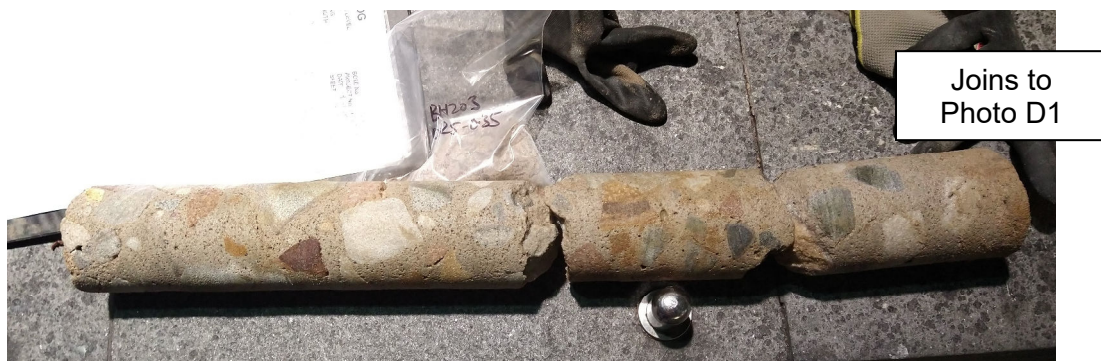
Photo D1 – View of top part of concrete core from Borehole BH203, showing a cemented coarse sand matrix between 0.02-0.09 m over a concrete slab. Reinforcement steel (9 mm diameter) was encountered in the lower part of the slab at 0.22 m depth.
