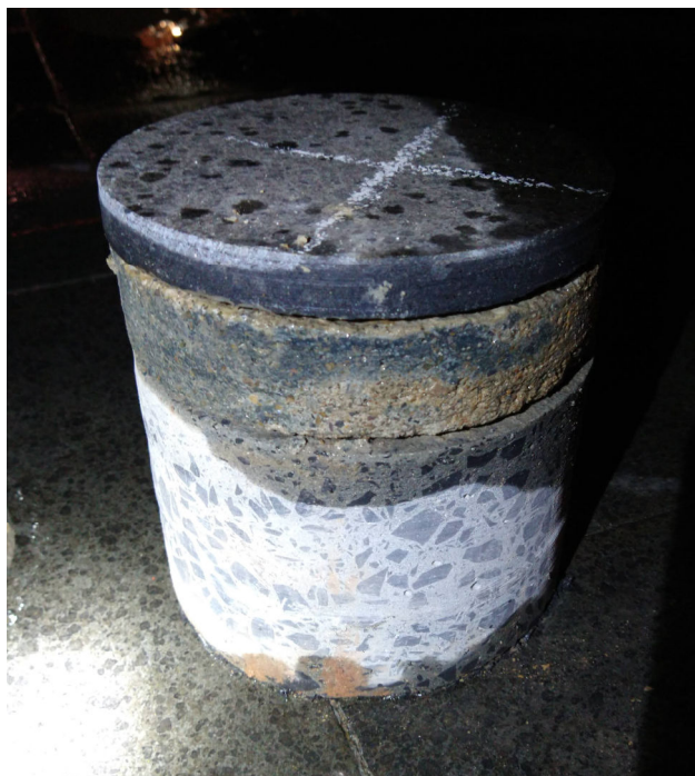
Photo D14 – View of concrete core obtained from Borehole BH1007. Steel reinforcement was observed within the concrete slab at 0.14-0.15m depth.
