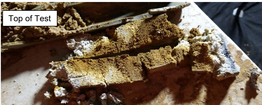
Photo D18 - SPT test from Borehole BH1007, depth interval 7.0-7.45m. The top of test indicated as shown.
