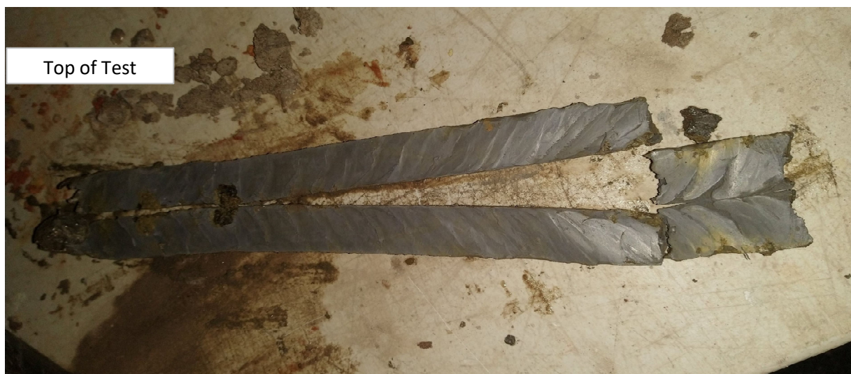
Photo D9 - SPT test from Borehole BH1005, depth interval 5.5-5.95m. Top of test indicated as shown.
