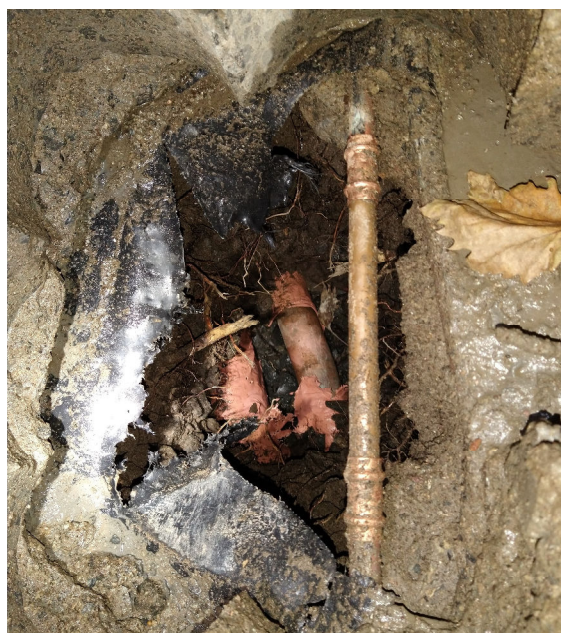
Photo D13 – View of two more deeply buried copper pipes within Borehole BH1006, at the termination depth of 0.8m.
