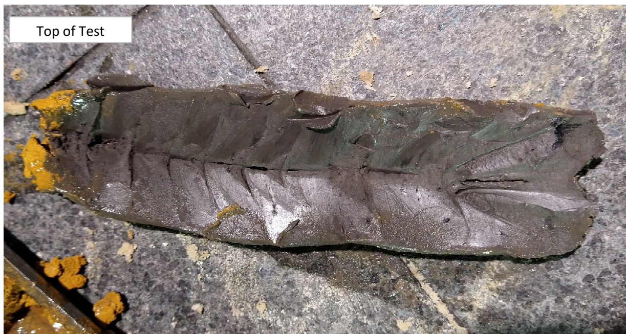
Photo D6 - SPT test from Borehole BH1004A, depth interval 4.5-4.95m. Top of test indicated as shown.
