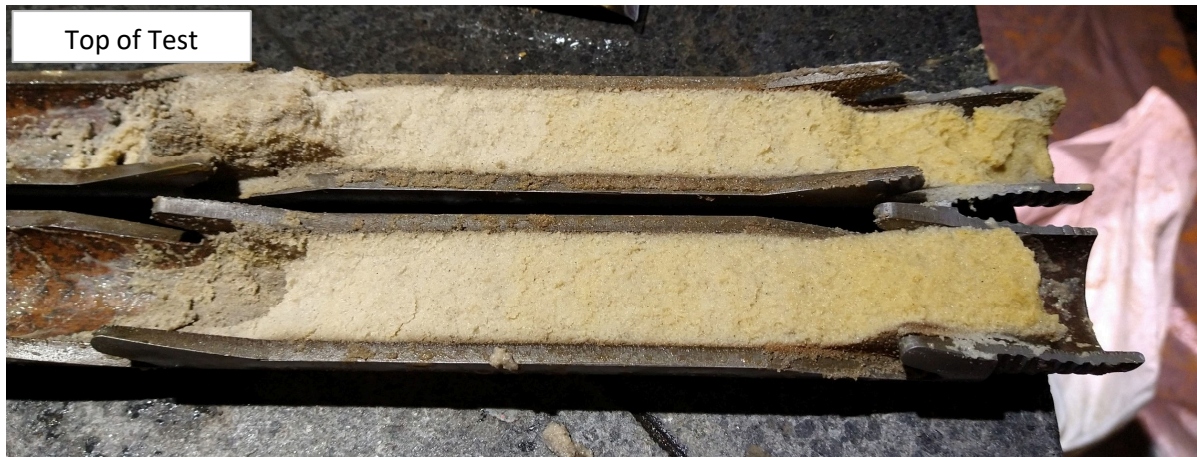
Photo D4 - SPT test from Borehole BH1003A, depth interval 2.5-2.95m. Top of test indicated as shown.
