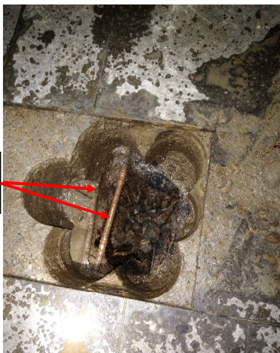
Photo D12 – View of copper water pipes and igneous rail ballast rubble beneath the surface at Borehole BH1006.
