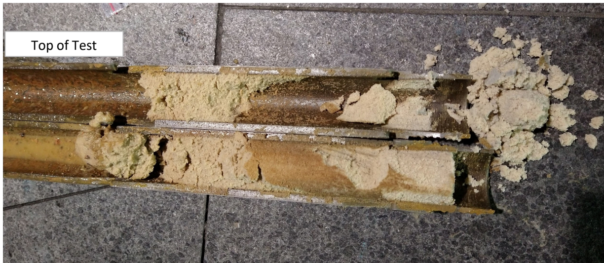
Photo D5 - SPT test from Borehole BH1004A, depth interval 3.1-3.55m. Top of test indicated as shown.
