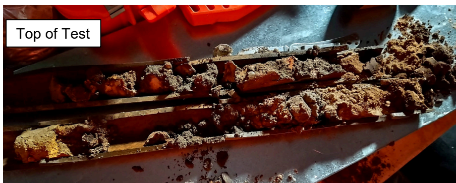
Photo D15 - SPT test from Borehole BH1007, depth interval 2.5-2.95m. The top of test indicated as shown.
