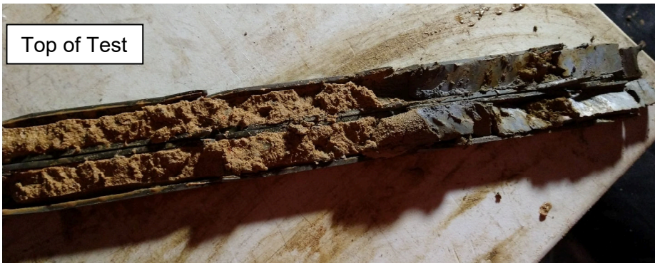
Photo D17 - SPT test from Borehole BH1007, depth interval 5.5-5.95m. The top of test indicated as shown.
