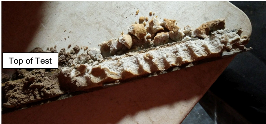
Photo D16 – SPT test from Borehole BH1007, depth interval 4.0-4.45m. The top of test indicated as shown.
