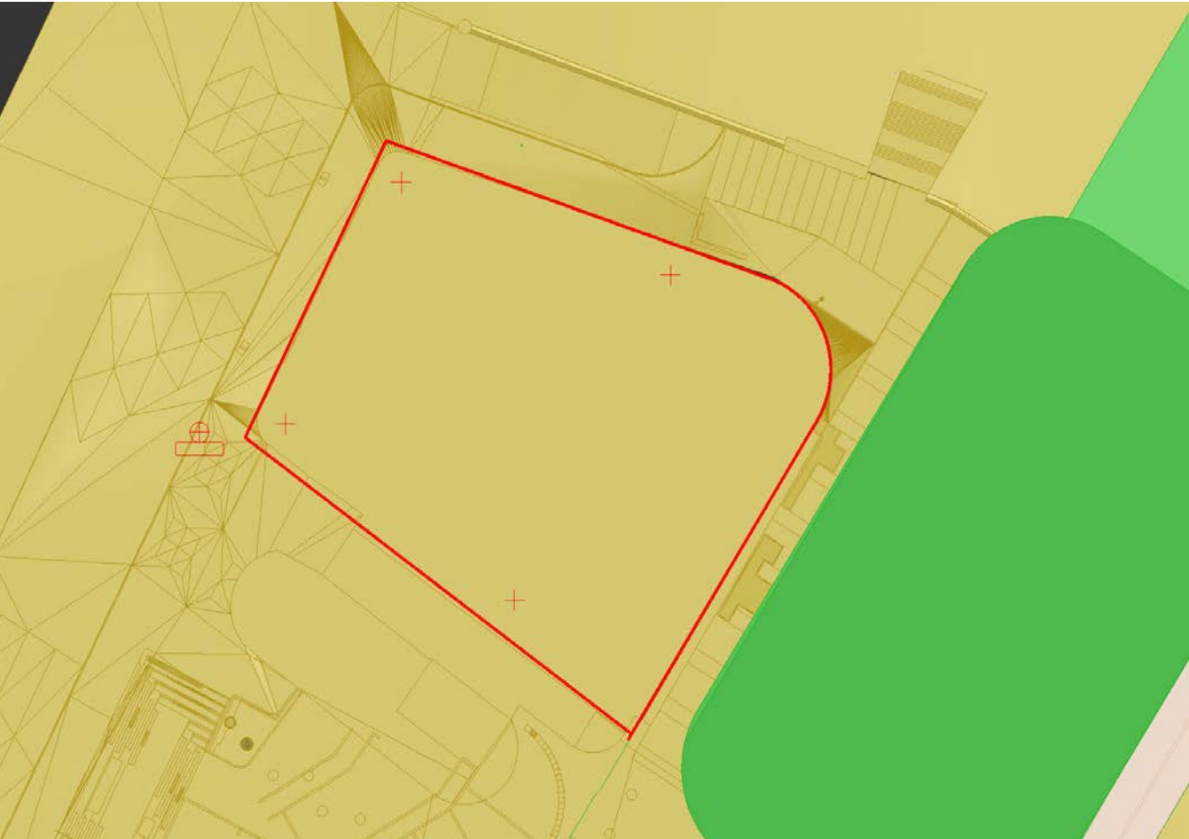
Image showing site boundary of 2 Lee Street from 3d Model (Yellow) aligned to survey drawing from Norton Survey Partners(Red Lines).
