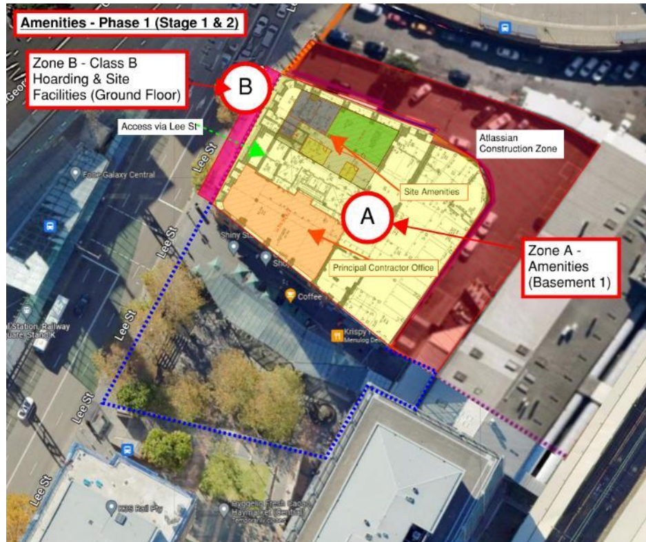
Figure5.3.2a – Phase 1 (Stage 1 & 2): Site establishment and early works
