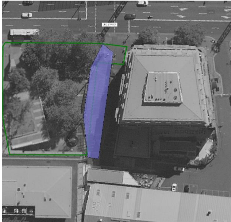
Figure 4.2.2a – Plan view of awning and south retail demolition works shown in purple.
