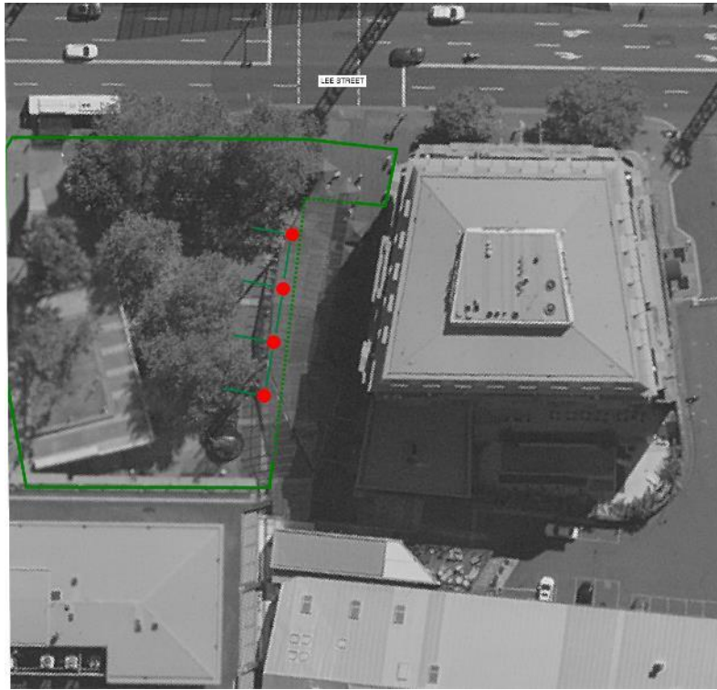
Figure 4.4.4a – Plan view of HDP megacolumn locations shown in red.
