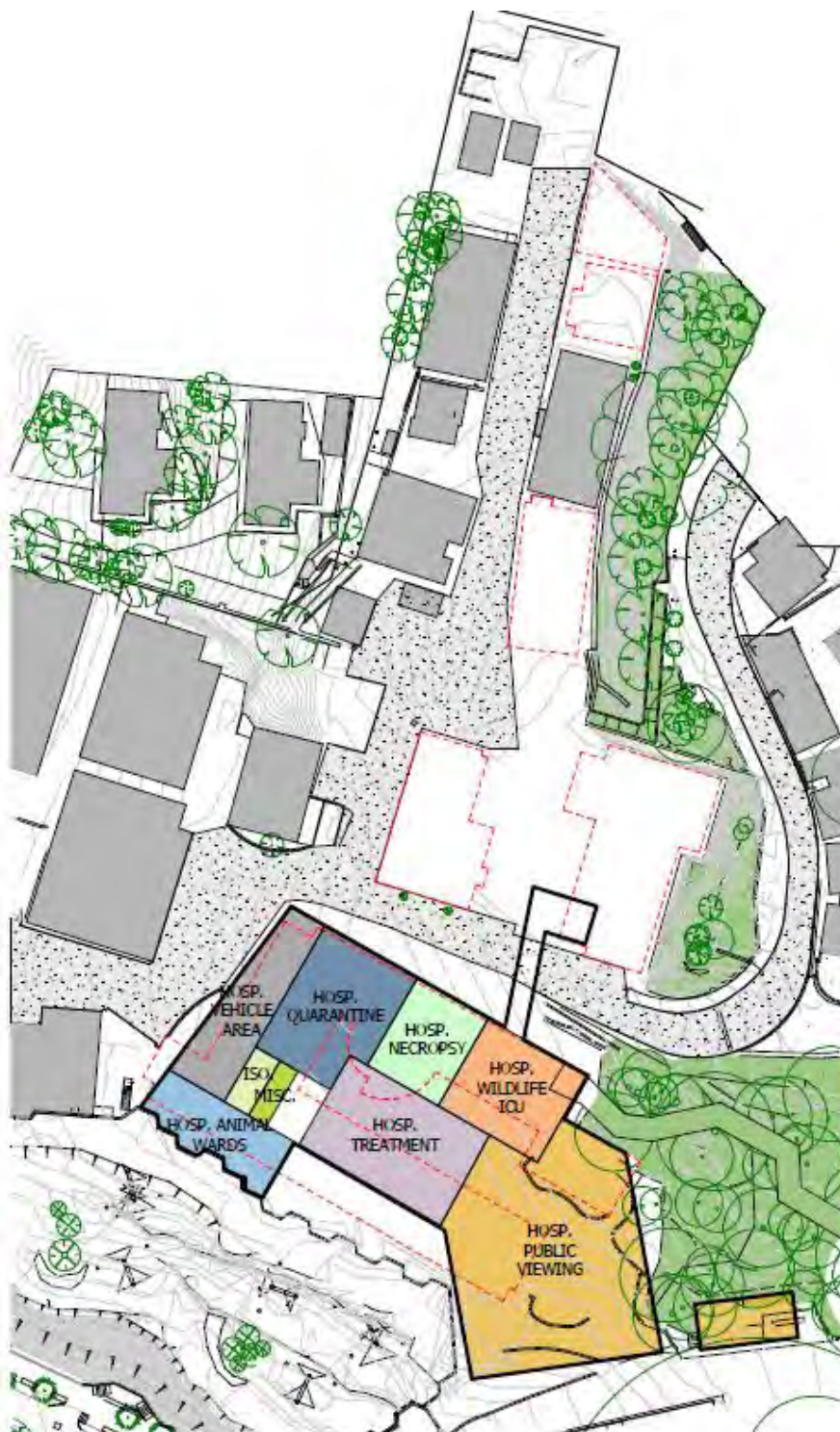
Figure 2 – Proposed building footprint and demolition plan.
