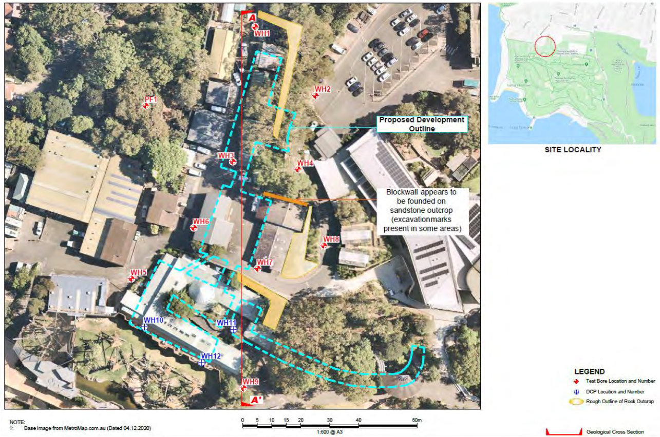
Figure 12 – Geotechnical Investigation – Borehole locations. Source: Douglas Partners, 2021.
