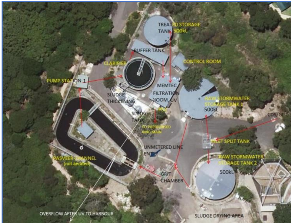
Figure 4.1 Waste Water Treatment Plant at Taronga Zoo
