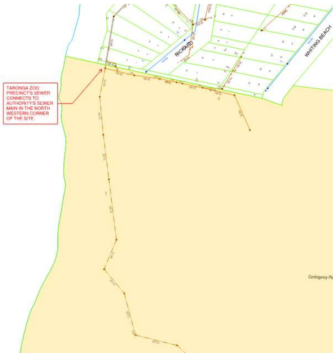
Figure 3– Precinct's Authority Sewer main connection.
