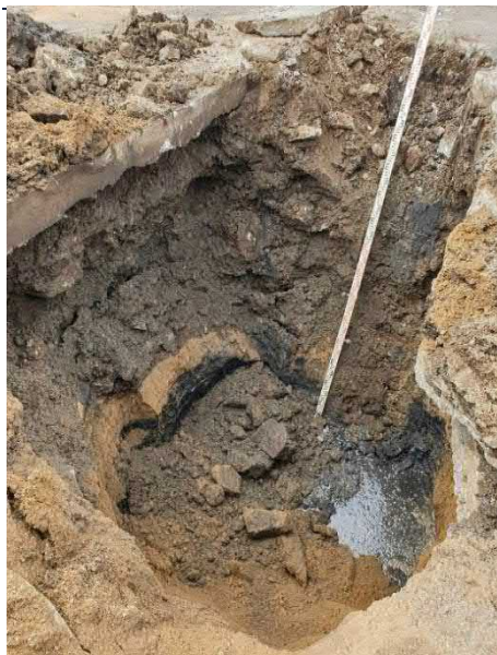
Photo 3-1 TP13 – Dark grey sandy clay Unit 3 (Estuarine) layer observed at 2.0-2.2m
