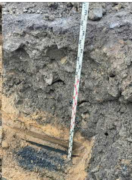
Photo 3-5 Example of dark grey clayey sand Unit 3 (Estuarine soils) approximately greater than Unit 1 (fill) and Unit 2 (Aeolian) layers sand
