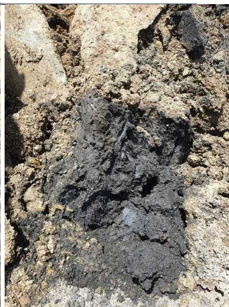
Photo 3-3 TP14 – Dark grey sandy clay Unit 3 (Estuarine) layer observed at 1.2-1.4m
