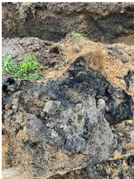
Photo 3-4 Example of dark grey clayey sand Unit 3 (Estuarine soils) approximately greater than 2.2 m bgl.
