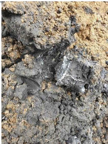
Photo 3-2 TP13 – Dark grey sandy clay Unit 3 (Estuarine) layer observed at 2.0-2.2m
