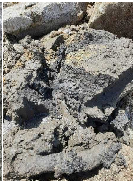
Photo 3-6 TP14 Clayey sand, pale grey Unit 3 (Estuarine soils) approximately greater than 2.4 m bgl.
