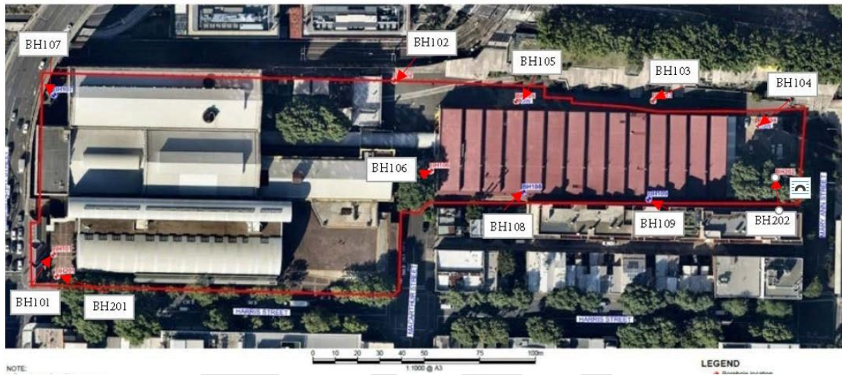
Figure 4-16: Location of geotechnical boreholes associated with the study area. Harris Street runs horizontally along the bottom of the image and Mary Ann Street runs vertically at the right-hand side of the image (Source: Douglas and Partners: Appendix B)
