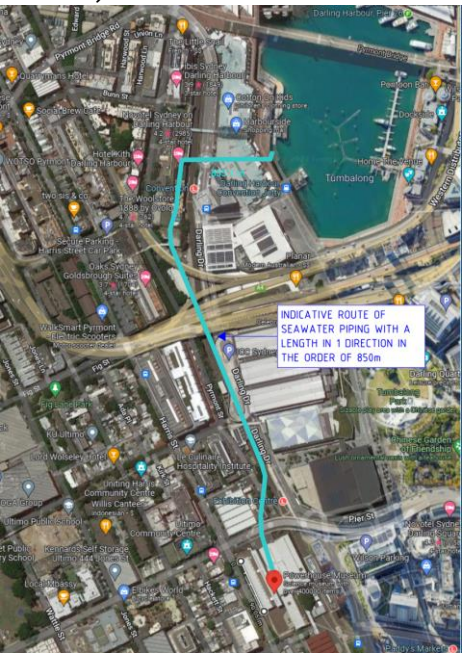
Image 1 : Indicative route of the existing Seawater Tunnel
