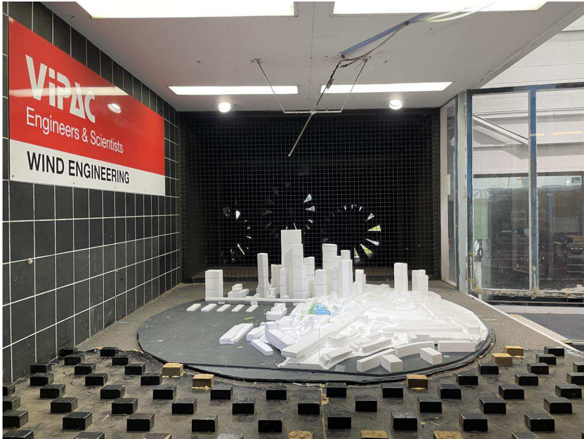
Figure 4: Overall view from north of the 1:400 scale model of the proposed development in the wind tunnel.
