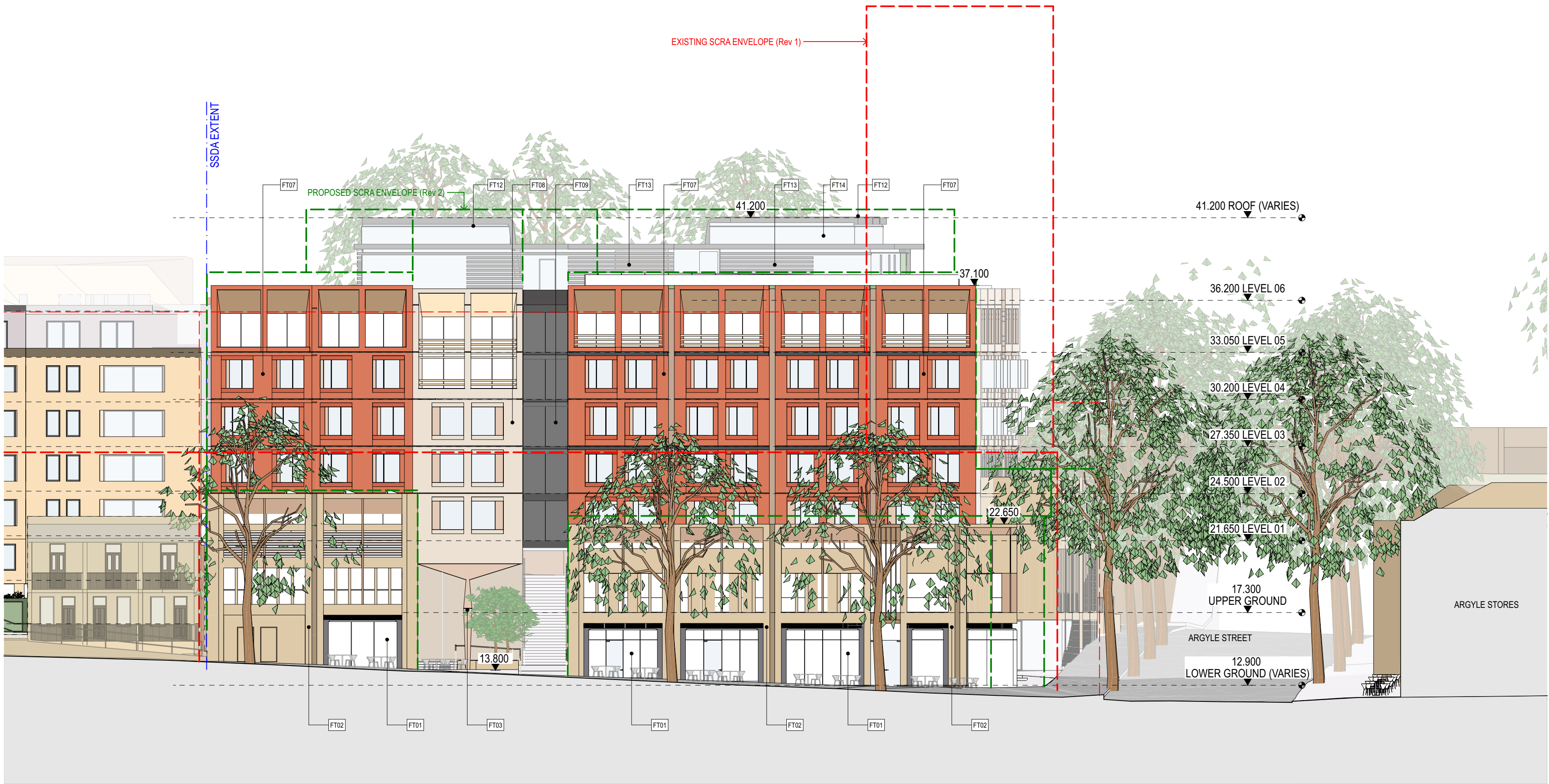
1 ELEVATION Harrington Street Elevation 1:200
