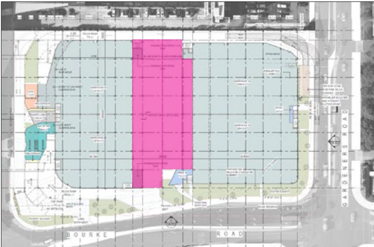
Figure 14 All-weather access and staging area
