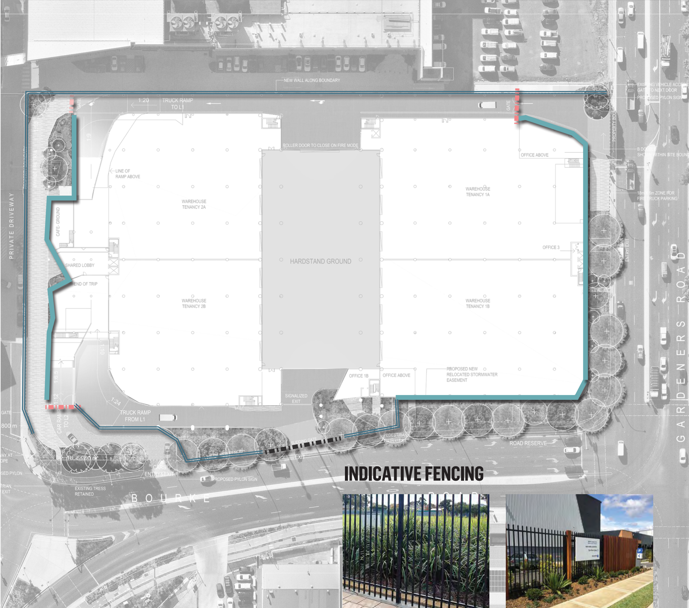
2.1m High fixed palisade fence set back 1.5m to allow planting next to footpath
