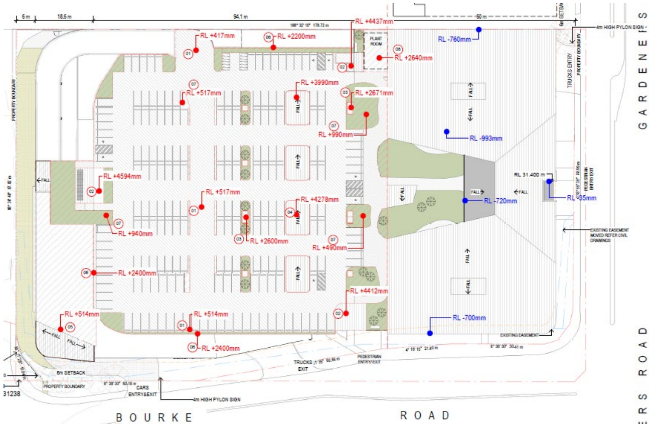
Figure 7 Height Control Blanket Diagram
